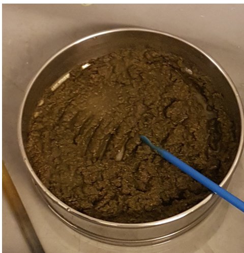
Fig. 3.1. As received diatom frustules, after being drained.
