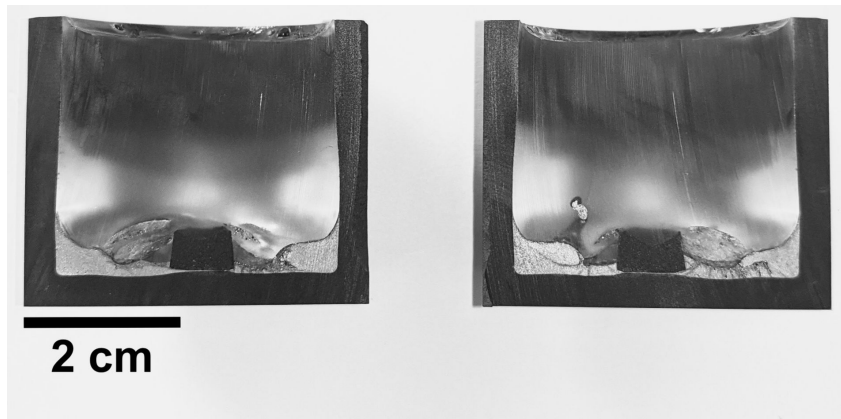
Figure 77: Crucible after the first cutting, from experiment M4 where quartz A was heated to 1950 °C for for 60min.
