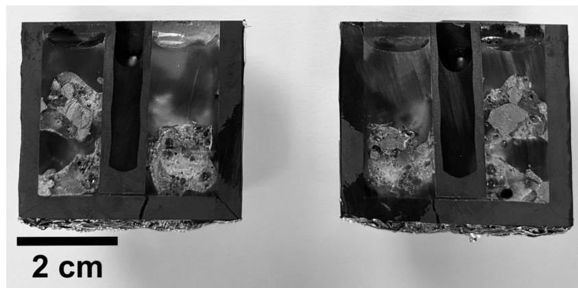
Figure 75: Crucible after the first cutting, from experiment M1 where quartz A was heated to 1750 °C for for 120min.
