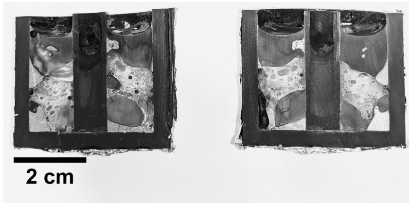
Figure 76: Crucible after the first cutting, from experiment M3 where quartz A was heated to 1850 °C for for 60min.
