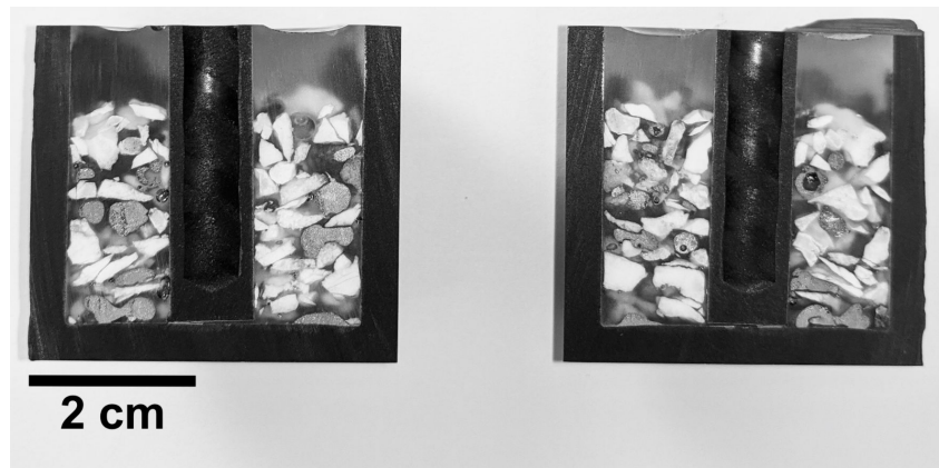
Figure 74: Crucible after the first cutting, from experiment M2 where quartz A was heated to 1650 °C for for 120min.
