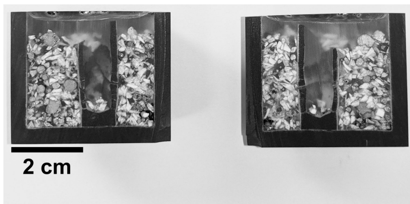
Figure 78: Crucible after the first cutting, from experiment M5 where quartz B was heated to 1650 °C for for 120min.
