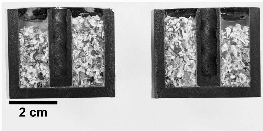
Figure 86: Crucible after the first cutting, from experiment M6 where quartz E was heated to 1650 °C for for 120min.
