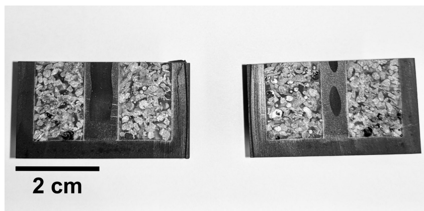
Figure 80: Crucible after the first cutting, from experiment M14 where quartz C was heated to 1650 °C for for 120 min.
