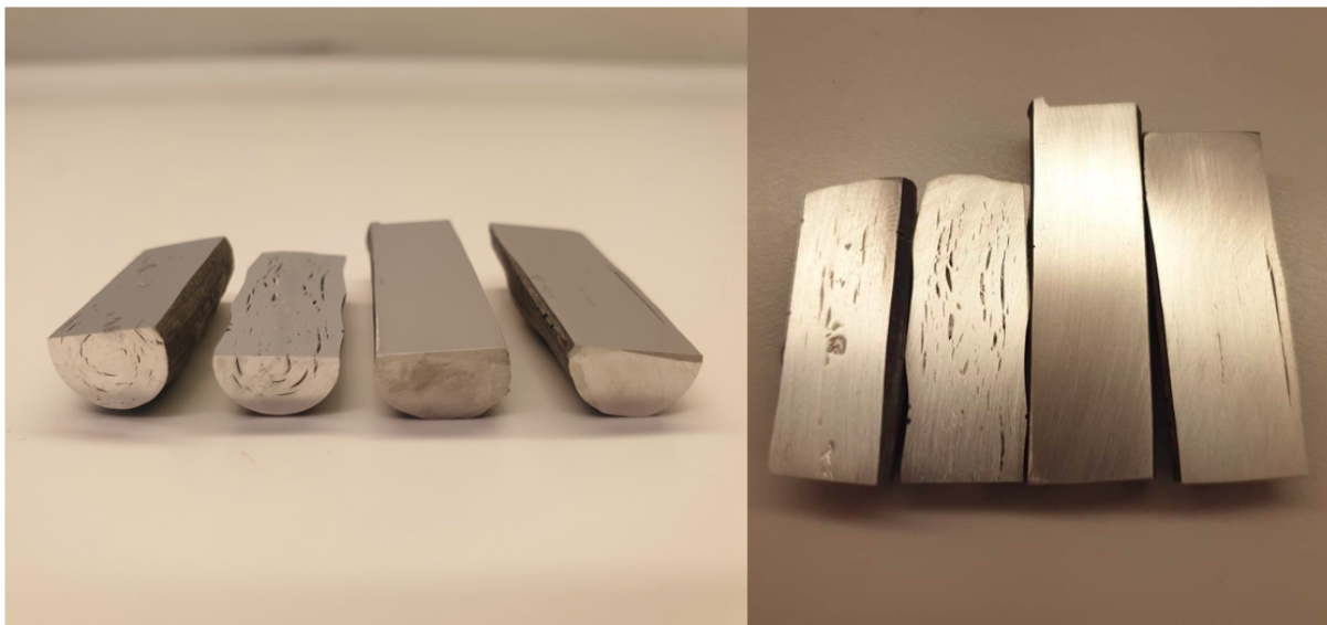
Figure 4.1: Image shows transversal and longitudinal cross-sections of metal continuous screw extruded (MCSE) 10 mm extrudate profiles. The extrudates were held at 560 °C for 2h in inert argon atmosphere. Leftmost, AA5183-CG, then AA5183, AA5183TiC-CG and AA5183TiC. Profiles extruded using CO 2 cover gas are labeled "CG". The samples are approximately 1-2 cm in length.
