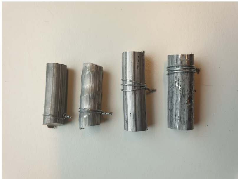
Figure 3.4: From left the first sample is AA5183-CG, second sample AA5183, third sample AA5183TiC-CG and fourth sample AA5183TiC. The steel wires were used to indicate sample number. Extrudates produced by Ragnvaldsen [12].
