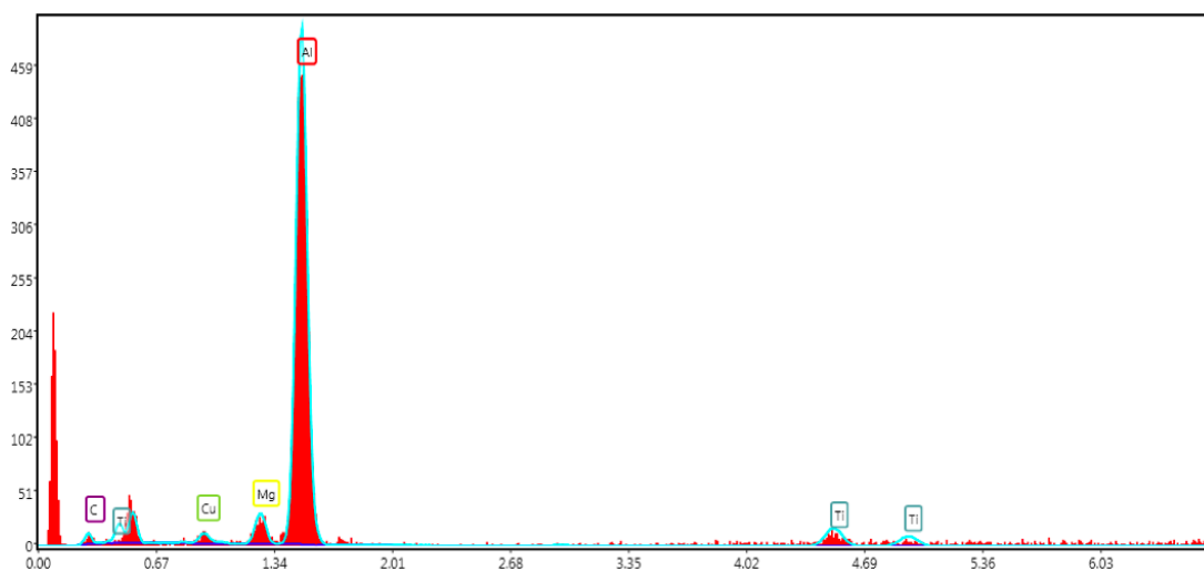
Figure 7.3: EDS point analysis of white particles in Figure 4.14, assumed to be clustered TiC nanoparticles.
