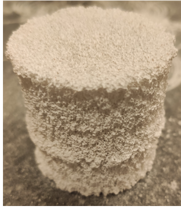
Figure 5.8: A sample of Sivex 80. Note the ridges around the middle.
