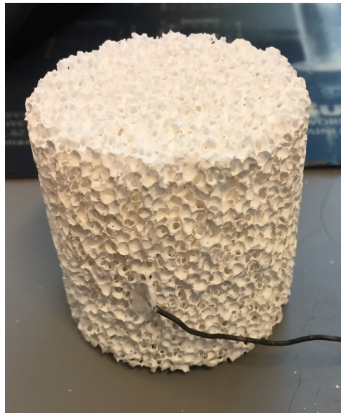
Figure 4.4: A sample with a thermocouple wire attached.
