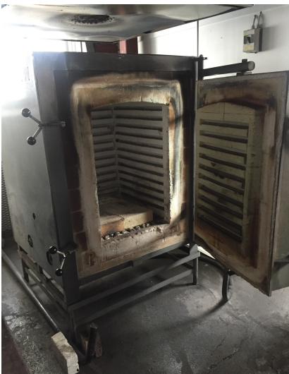
(c) Oven used for drying the samples after cutting and prior to compression test.
