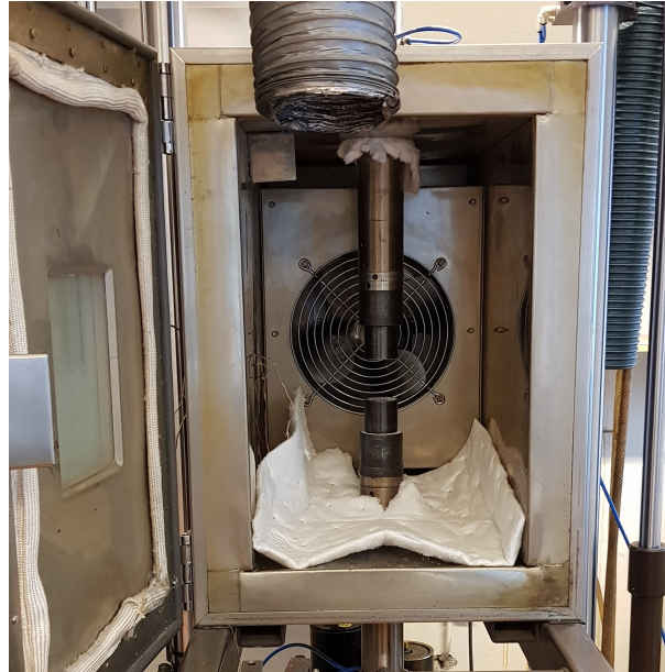
Figure 4.1: The MTS 880 Hydraulic Tensile Testing Machine 100 kN.
