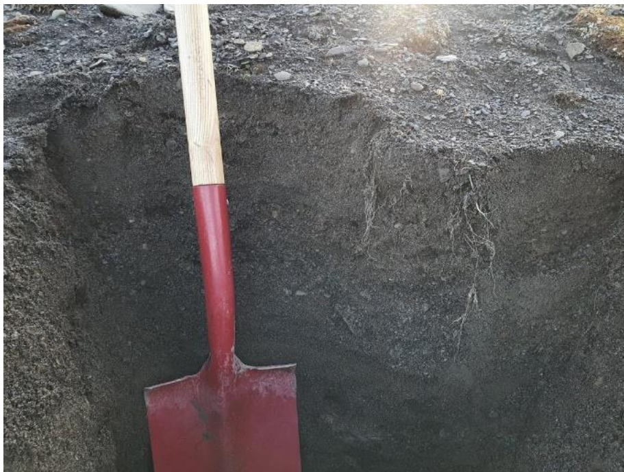
Figure 19: Picture of the cross section nr 10 (for location see fig 18). Different layers of coarse sand and gravel is observed with some larger cobbles imbedded. More information about this cross section can be found in the appendix. Photo: Vendela Hergot.
