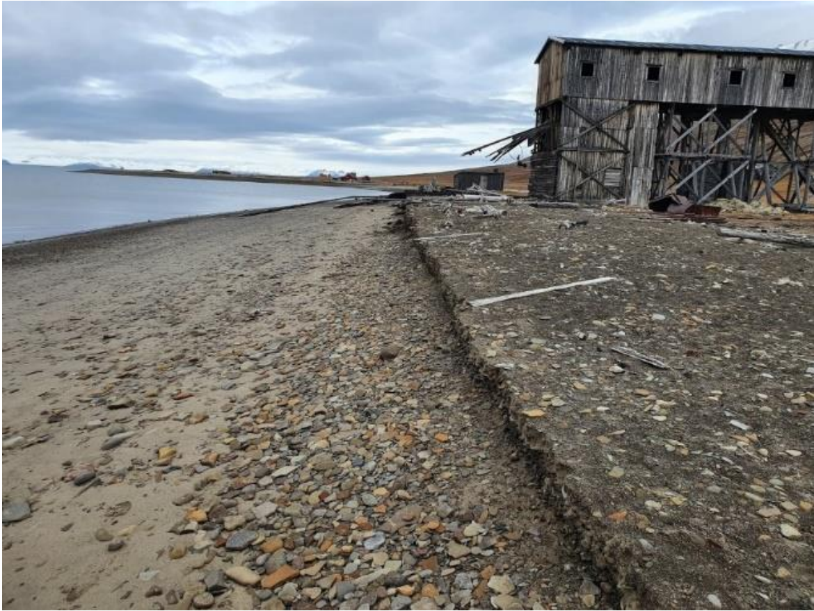
Figure 11: The erosion edge seen in figure 6 is an example of an erosional edge that was followed when mapping. When walking with the Gtac or handheld GPS the point was taken just above the erosion line. Photo: Vendela Hergot
