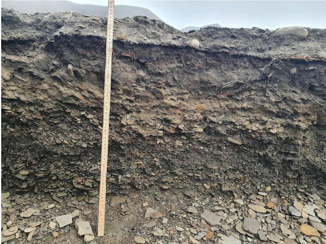
Figure 28: Cross section nr 1 at Hiorthamn, for location see fig 26. This cross section show different stratified layers of sediment, and sediment samples were taken from the four layers close to the surface.
