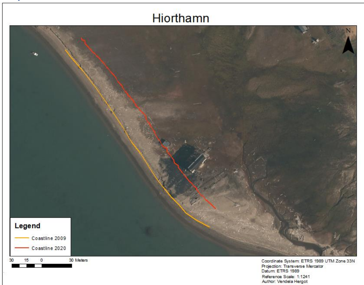
Figure 24: Changes along the coastline of Hiorthamn between 2009 and 2020. The basemap in this figure was taken by NPI (2009). The red line represents GPS points that were taken along the active spit during fieldwork in the fall of 2020, the yellow line traces the spit present in 2009.
