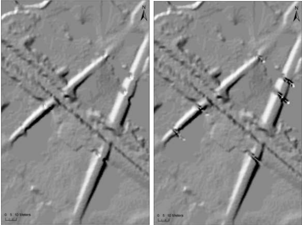
Figure 12: Hillshade before and after manipulating the culverts
