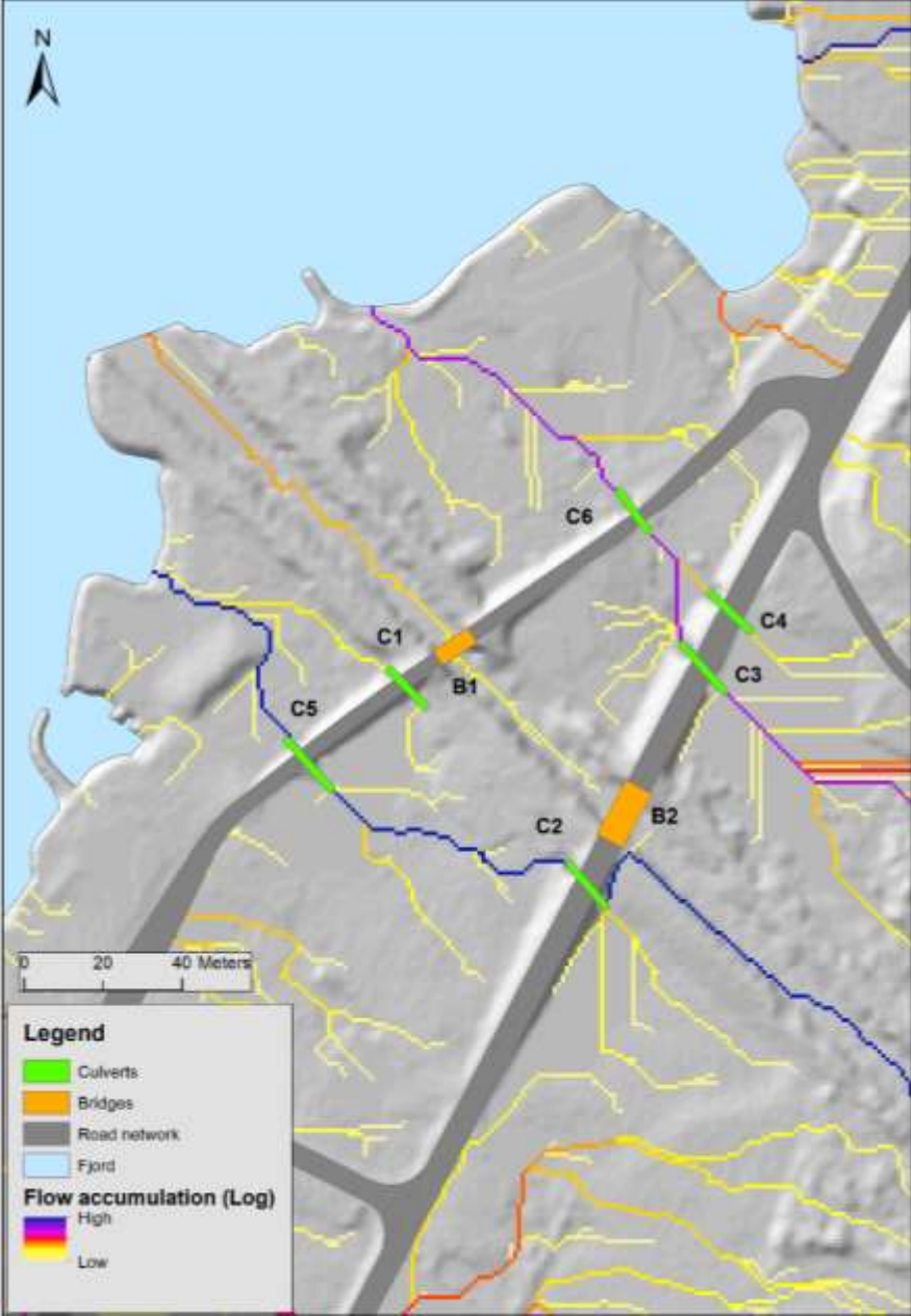
Figure 28: Flow accumulation when B2 is closed & all culverts are open
