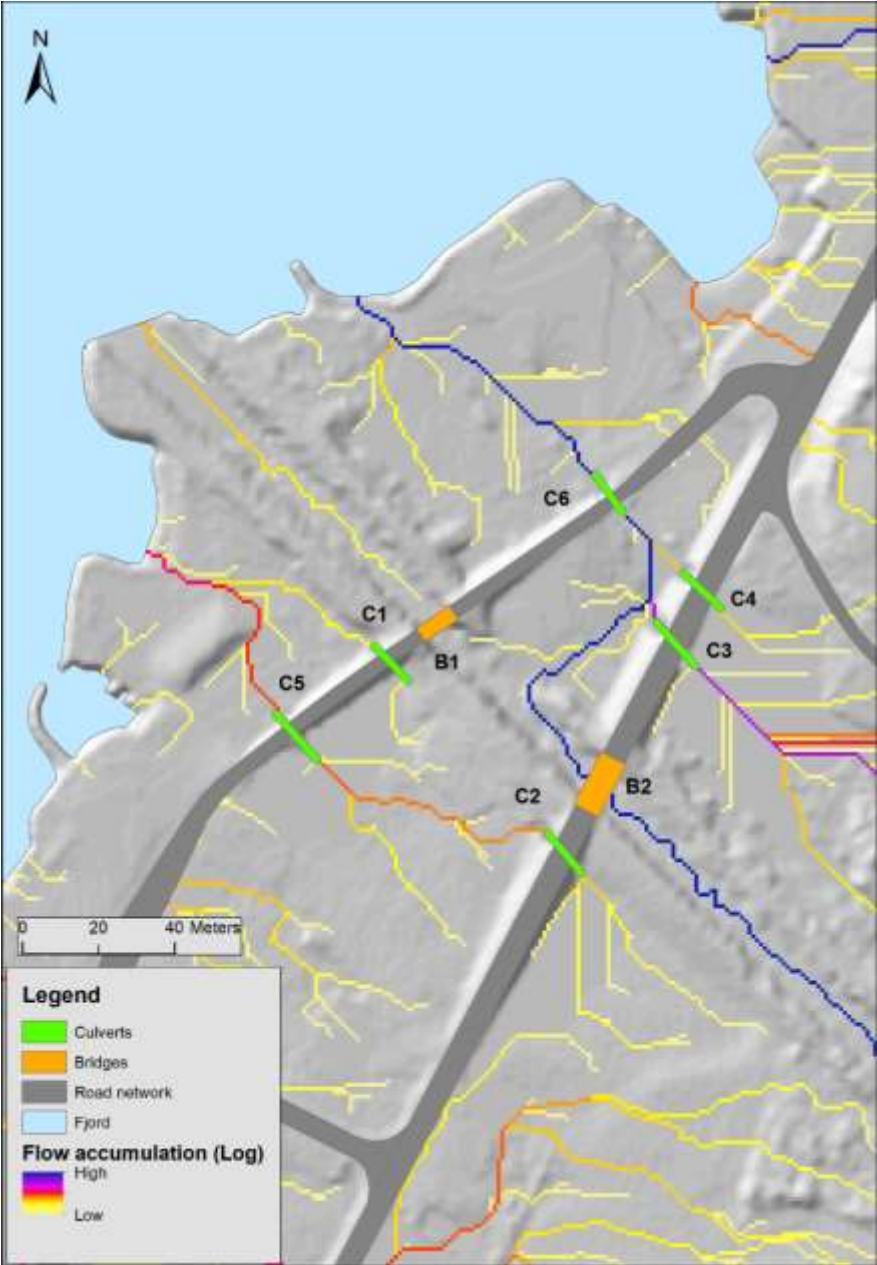
Figure 26: Flow accumulation when B1 is closed & all culverts are open
