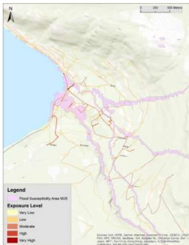
Figure 61: NVE susceptibility map compared to the resulted mean road segments exposure map of all scenarios
