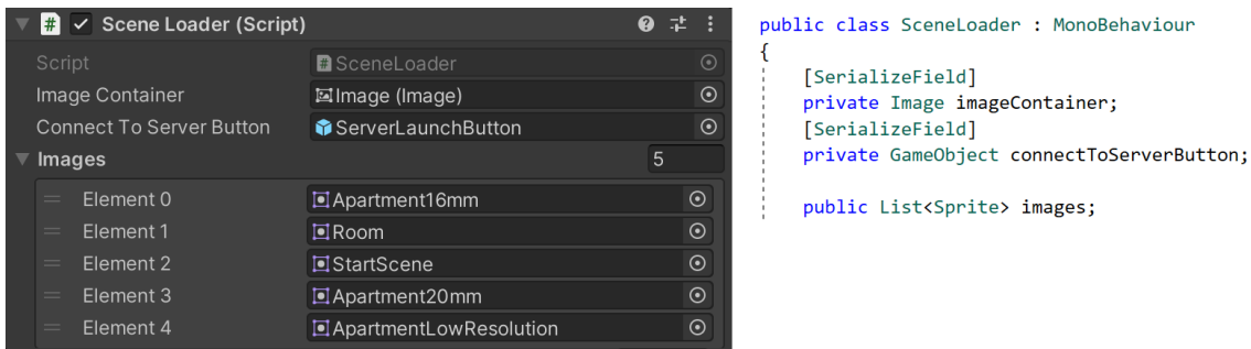
Figure 2.9: Variables in a script that inherits from MonoBehaviour and is made adjustable in the inspector. All public variables are automatically adjustable in the inspector in addition to private variables with the tag [SerializeField] .
