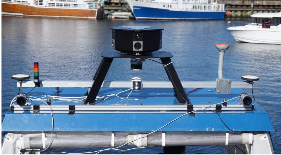
Figure 4.5: The sensor rig in black while the stereo rig is provisionally mounted on the roof of the ferry
