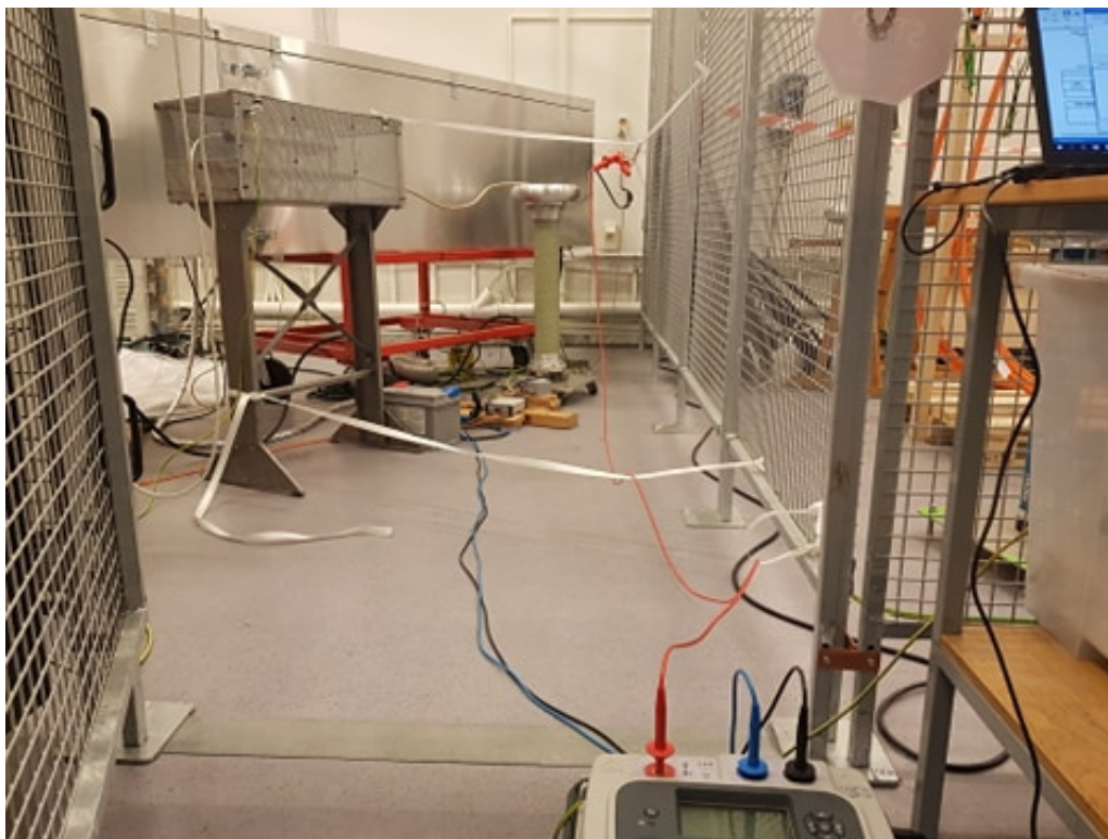
Figure 10: Overview of the test cell. The large silver box on the left side holds the generator bars and will maintain temperature at the desired level. A significant amount of the equipment is used in the other project.
