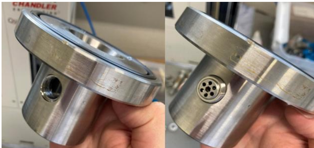
Figure 5 The Pressure Cell Used in the HP Test Bench Before Inserting a Valve (Left) and with an Injection Valve Inserted (Right)
