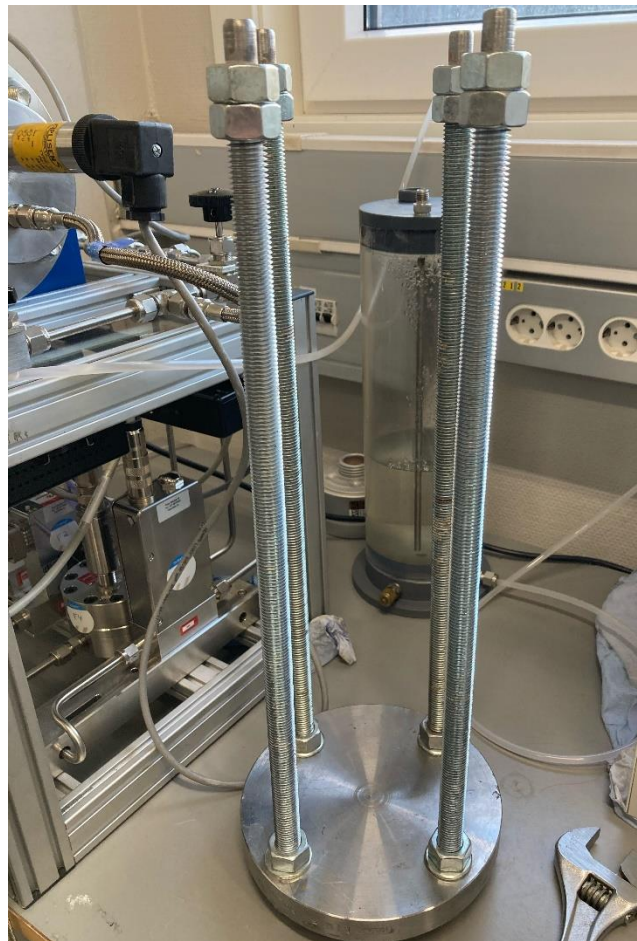
Figure 55 Stand Used to Hold the Pressure Cell When Changing Valves
