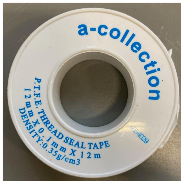
Figure 57 Thread Seal Tape Used to Decrease Thread Leakage
