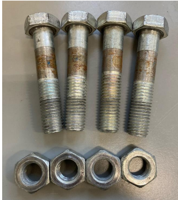
Figure 52 Bolts and Nuts Used to Keep the Pressure Cell in Place
