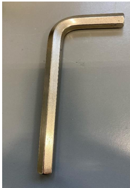
Figure 53 Key used to Insert the Injection Valves
