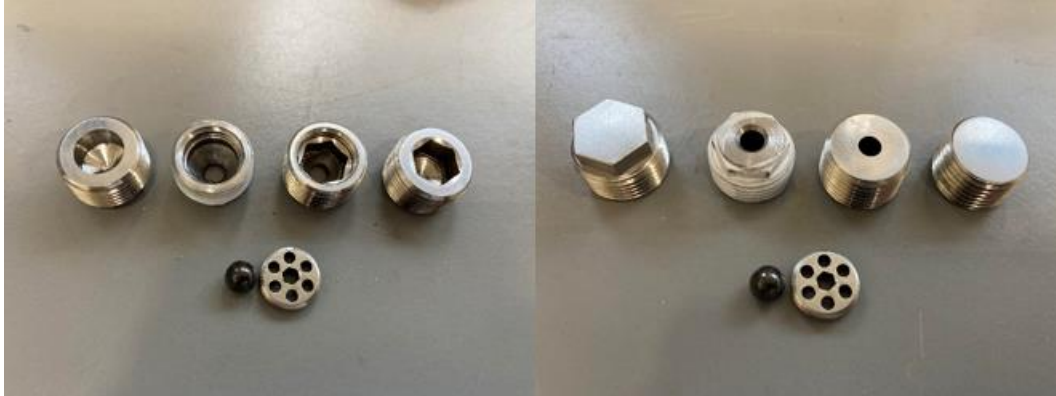
Figure 4 The Production Blind, Production Valve, Injection Valve, and Injection Blind (from left to right), with the Silicon Nitride Ball and the Hex-hole Lid Used (Top view and Bottom view)
