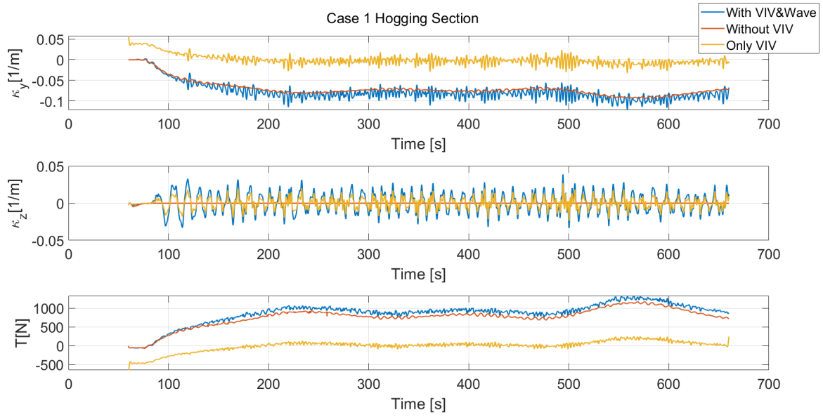
Figure 9.1.8: Global Analysis Results for Case 1 Hogging Section
