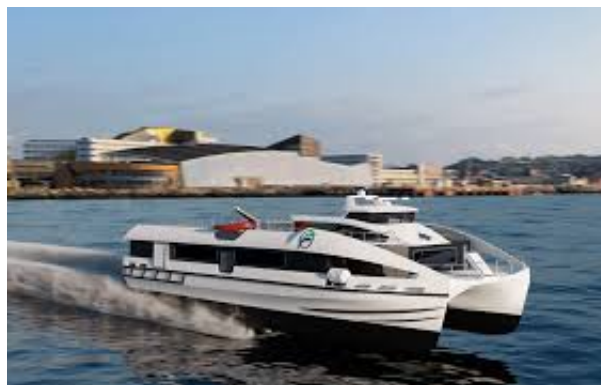
Figure 2.3: Illustration of one of the Flying Foil vessel solutions (Courtesy: Godø and Vinje (2019))
