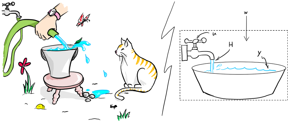
Figure 2.1: A model (right) is a simplified representation of reality (left). The dashed line represents the boundaries of the defined system.
