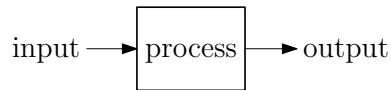
Figure 2.3: Block diagram representation of a system. Arrows represent signals and blocks represent processes.
