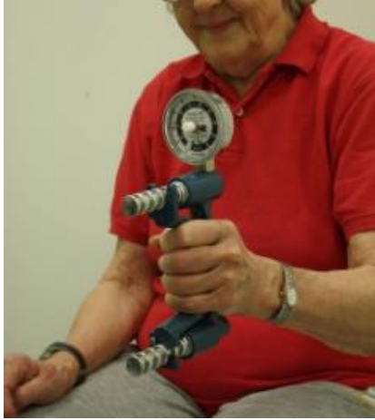
Figure 3: Illustration of a typical hand dynamometer and position for grip strength test.
