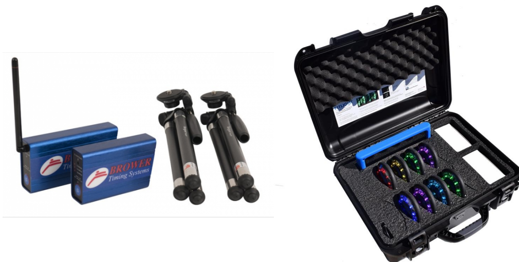
Figure 6 Brower timing system (left) and FitLight system (right) used for 40 m straight-line sprint and COD sprint testing, respectively.
