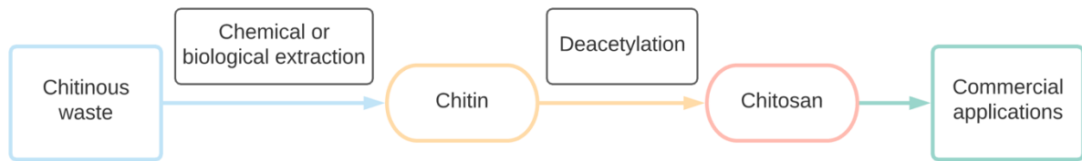
Figure 2.2 A scheme showing how chitin and chitosan can be extracted from chitinous waste by chemical or biological extraction, which further can be used for commercial applications.
