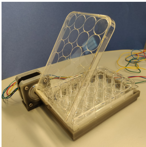
Figure 3.1: System for remote opening and closing of Corning Costar 24-well plate lid during UV sterilization protocol. The plate fits within the 3D-printed mount together with a SM-42BYG011-25 stepper motor screwed beside. An adaptor is slotted onto the stepper motor arm and super-glued to the plate lid. Using an Arduino Pro Micro, the plate lid can be raised and lowered at will.
