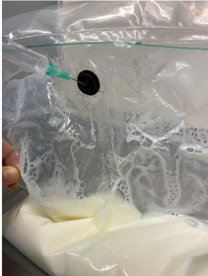
Figure 12: The placement of the rubber injection port at the headspace of the bag.
