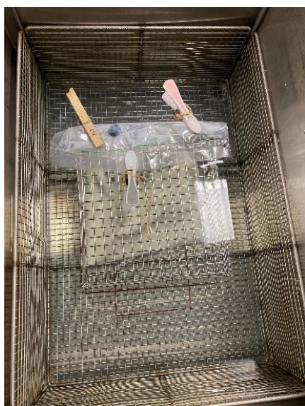
Figure 14: Detail of the sample pouch in the US bath. The pouch is placed approximately in the middle of the US bath (13.5 cm from short sides and 6.5 cm from the long sides) inside a metal cage.
