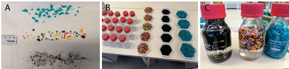
Figure 2.2: Plastic fragments from balloons (multiple colors), nitrile lab gloves (turquoise), and granulated car tire rubber (black). The photos display (A) plastic fragments from the three materials used for measurements of size distribution; (B) fragments divided into five containers with 40 g each, and (C) fragments and seawater combined in glass bottles.
