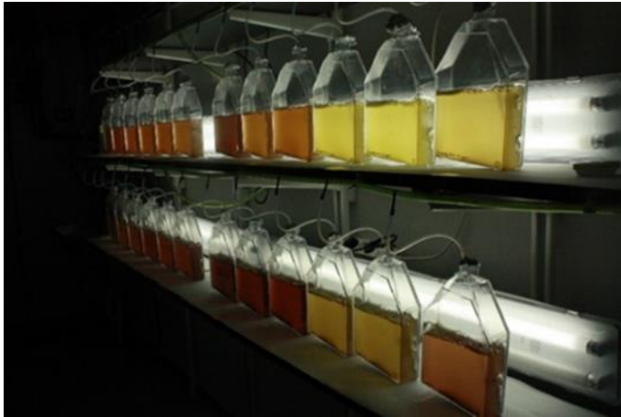
Figure 6: The two benches of culturing flasks. On the top bench the light intensity was higher than on the lower. The picture is taken during the culturing of R. baltica .
