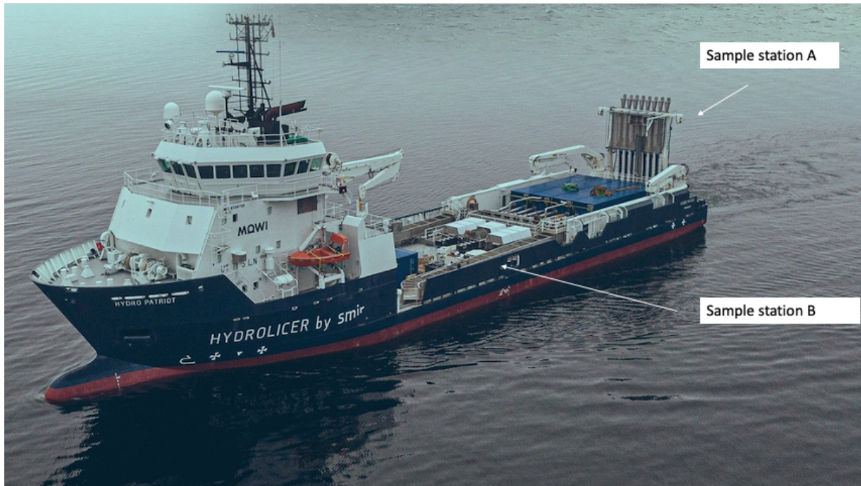
Figure 4 Hydro Patriot delousing vessel, where data was collected. Sample station A (pipes are elevated during sea travel) above the entrance of the Hydrolicer line. Sample station B at the water slide placed after Hydrolicer line.
