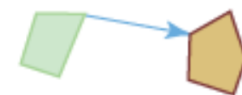
Figure 8 Illustration of where the shortest distance between two polygons is being calculated. Esri, 2019.
