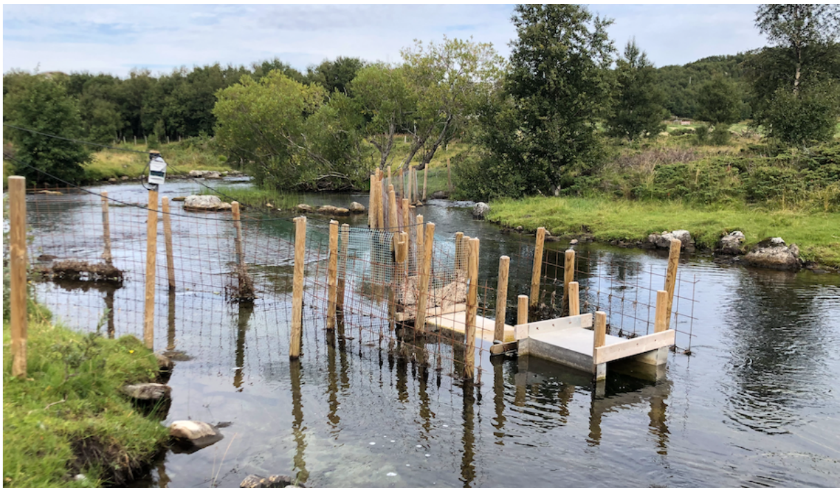
Figure 3: The video tunnel in river Fjæreelva with pit-antenna, guiding-fences, shade-cover and fences mounted on the side protect the tunnel from passing cows. The river flows from right to left. Picture was taken 21 August 2020.
