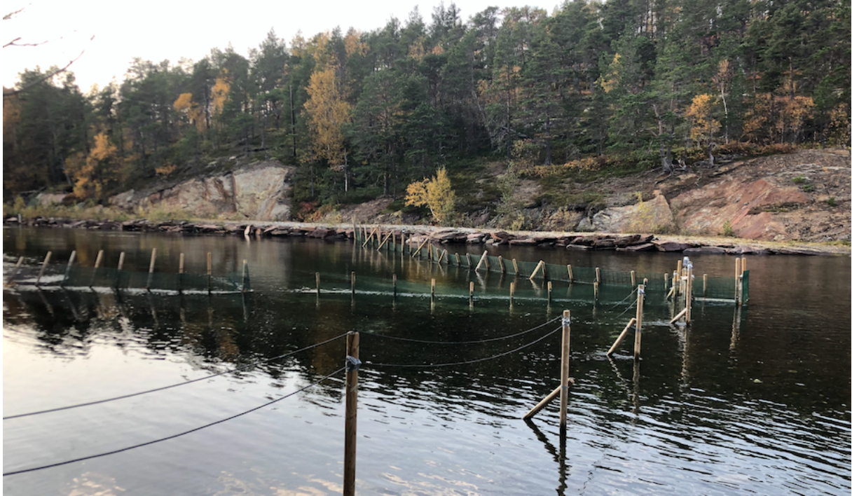
Figure 5: The video tunnel in river Botnelva with attached pit-antenna and guiding-fences. The river flows from right to left. Picture was taken 29 September 2020.
