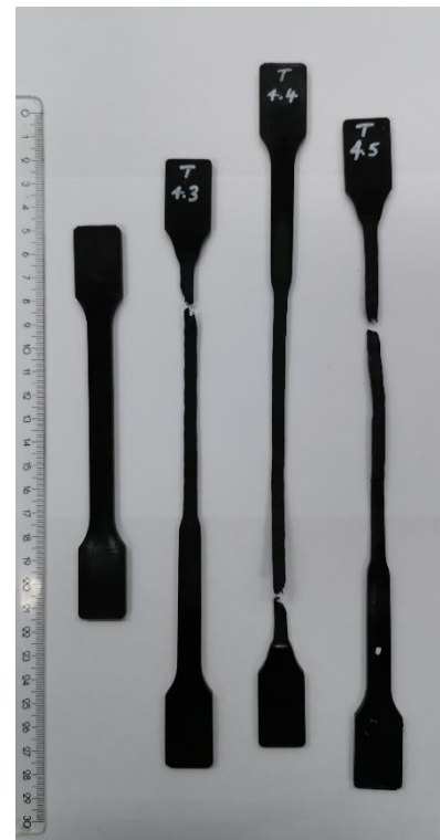
Figure 4.5: Tensile failure at 112 days
