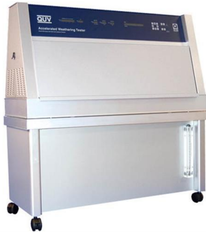
Figure 3.2: QUV Accelerated weathering tester (QLab, 2017).
