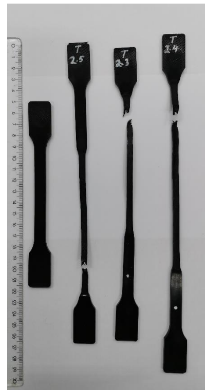
Figure 4.3: Tensile failure at 56 days
