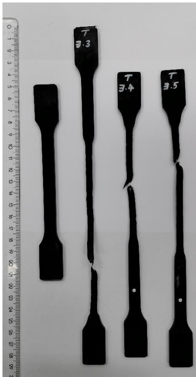
Figure 4.4: Tensile failure at 84 days
