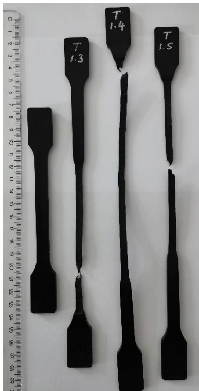
Figure 4.2: Tensile failure at 28 days
