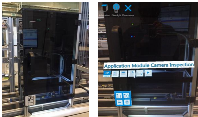
Figure 3. Camera station and the black and white augmented reality plug-in (on the left). The same station through the view of the Festo AR app (on the right).
