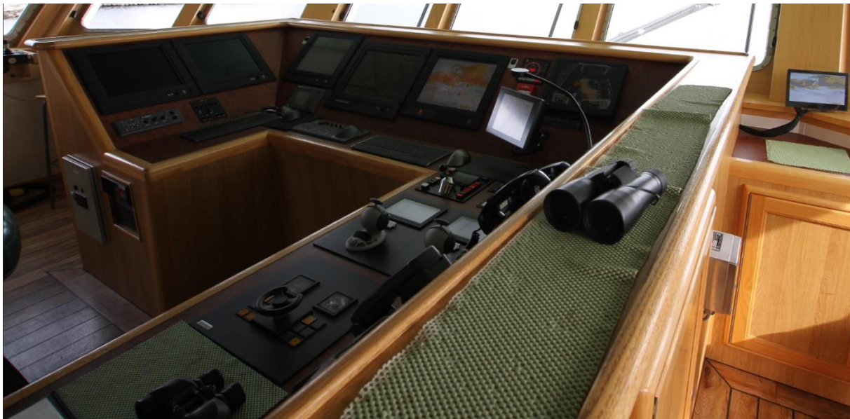
Figure 20: Photo of the console on Gunnerus bridge
