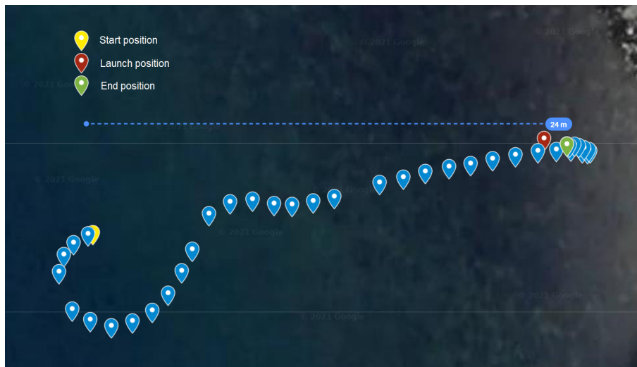
Figure 4.18: Path of the RTL autonomous mode
