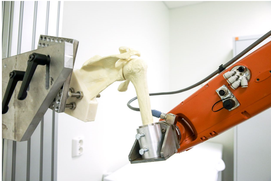
Figure 2.3: Kuka robot performing tests on a sholder joint.
