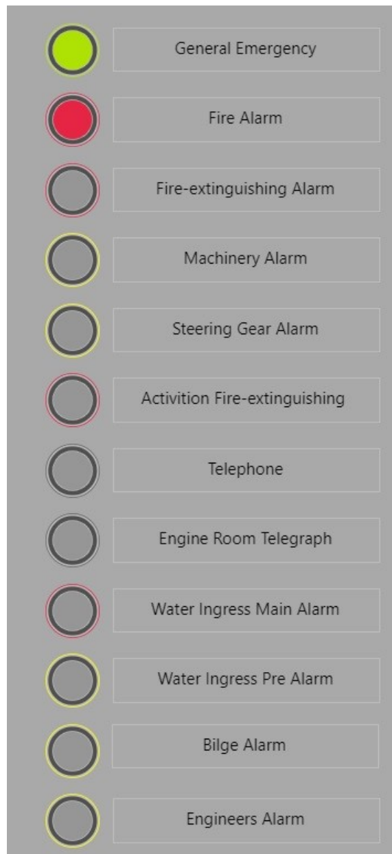
Figure 47: Alarm Panel with active alarms
