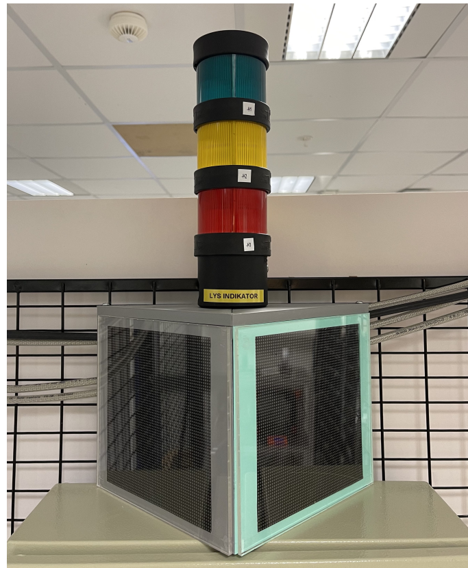
Figure 49: Prototype of PVS: Warning light on top, LED modules on bottom
