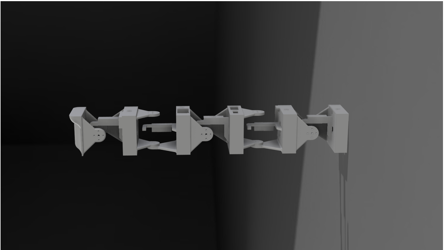
Figure 4.3: The snake-like robot without its LiDAR and equipment
