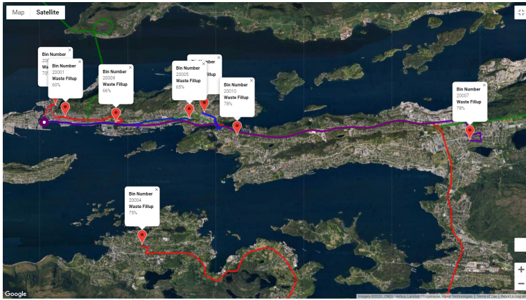
Figure 5.3: Optimized shortest routes with minimum distance through vehicle routing problem (VRP-distance)
