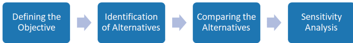
Figure 1: A overview of the basic principles of a trade-off study according to (Kossiakkoff et al. 2011)
