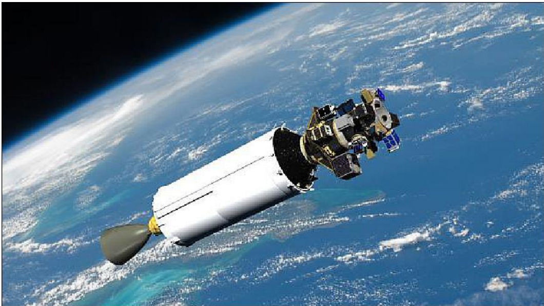
Figure 2-6: SSO-A Launch depiction with SpaceX Falcon-9 stage 2. A rideshare mission with 15 microsatellite and 49 CubeSats. (image credit: Spaceflight) [4]
