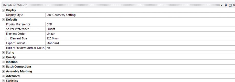
**Figure 72: Details of the global mesh.**
