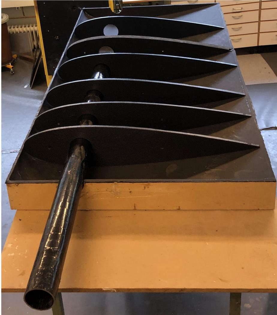
**Figure 51:** Mainsail with ribs and mast placed in the mainsail mould.
