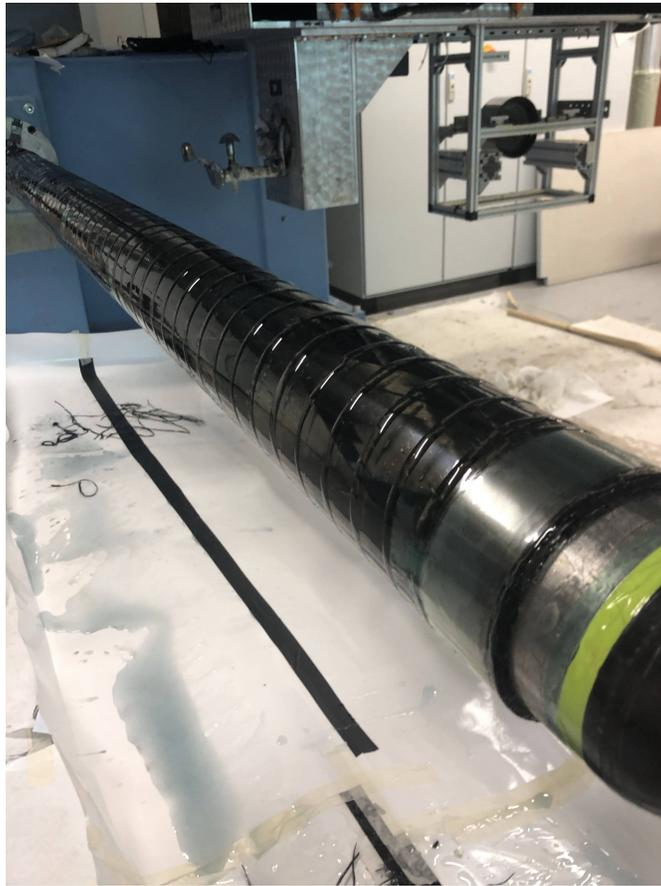
**Figure 36:** After the filament winding process was done with ends cut away and vacuum-bag strips attached.
