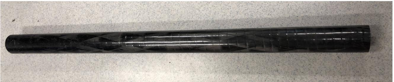
**Figure 54:** The CFRP mast with ends cutted.
