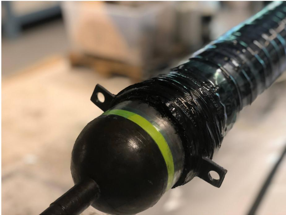
**Figure 37:** Illustration of the profiles attached to ease demoulding.
