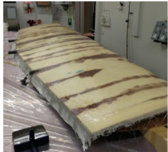
**Figure 1:** Wingsail produced as a sandwich structure with foam core [3].
