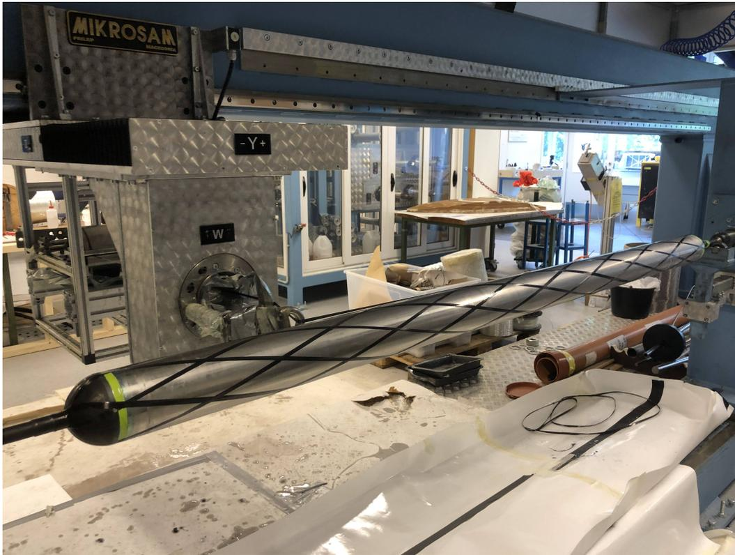
**Figure 35:** Start of the first layer of PAN carbon fiber wound onto the mandrel.
