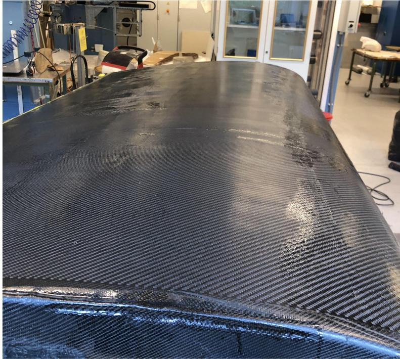
**Figure 53:** Mainsail shell after demoulding.
