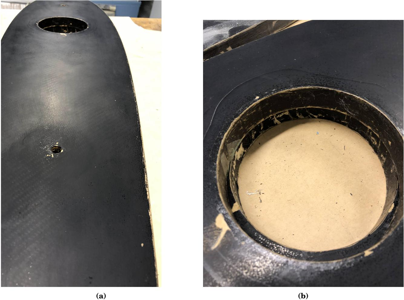
**Figure 57:** Some damage on the rib mould after demoulding was detected.
