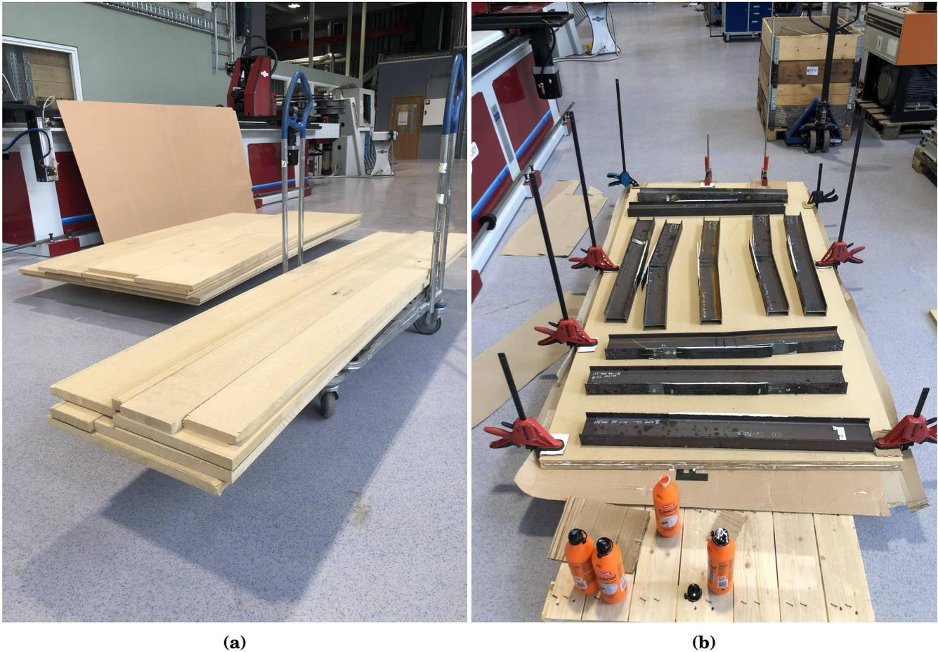
**Figure 25:** (a) Cutted MDF, (b) Gluing cutted MDF plates together with extra weights and clamps adding extra pressure.
