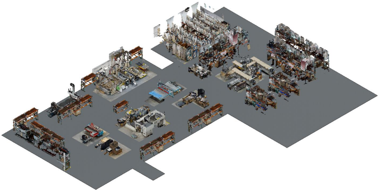
Figure 28. Detailed 3D model of the general overall layout with filtered and suppressed point cloud data.
