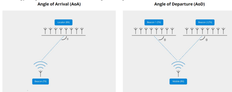
Figure 9: Illustration of the bluetooth 5.1 AoA and AoD method [7]
