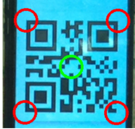
Figure 41: The vertices and the calculated center of the QR-code marked with circles.
