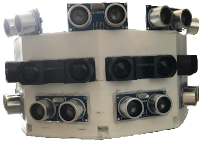
Figure 36: Obstacle detection grid consisting of ultrasonic and infrared sensors
