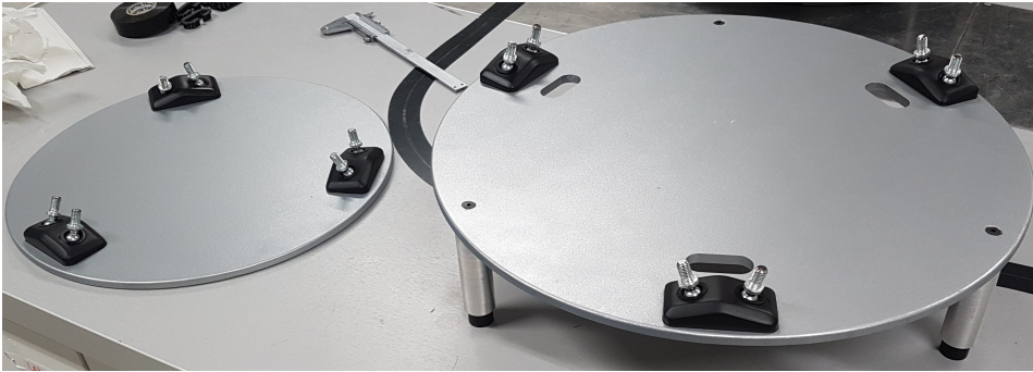
Figure 7.4: Produced top and bottom plates with brackets attached
