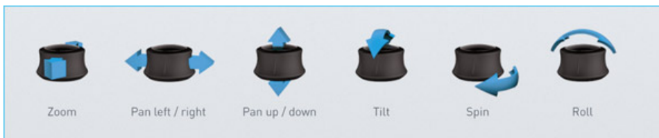
Figure 5.9: 3Dconnexion: Navigator cap and movements
