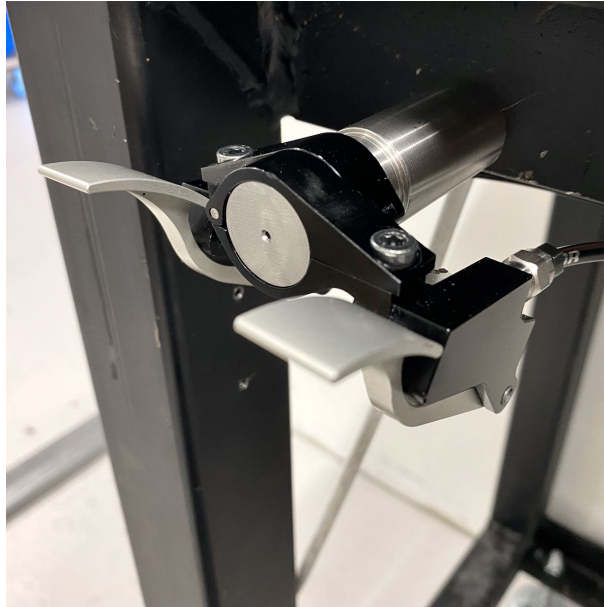
Figure B.7: Shifters for the Kindernay XIV mounted to the testing rig.
