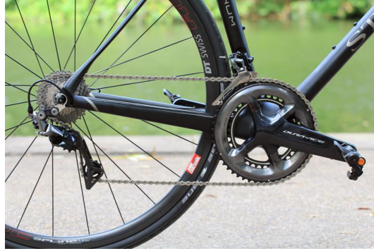
Figure 2.3: A chain-derailleur transmission on a road bicycle. Picture from road.cc [3].
