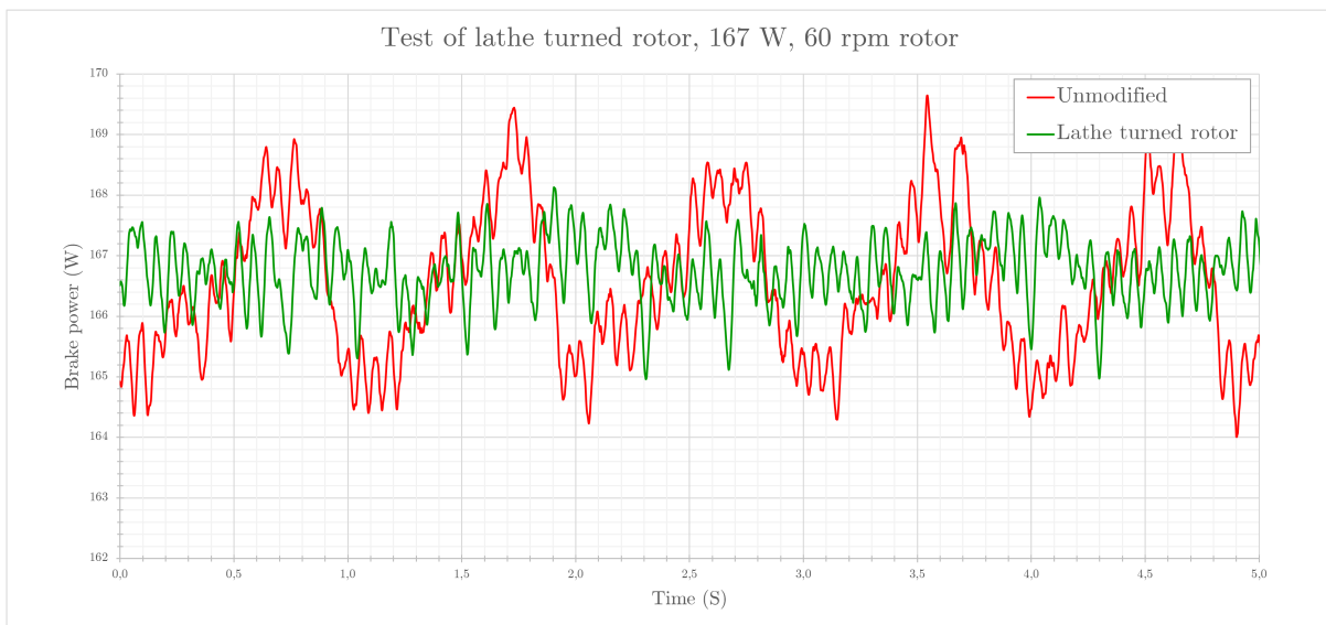
Figure 8.5: Comparison between the unmodified and lathe turned ECB rotor.
