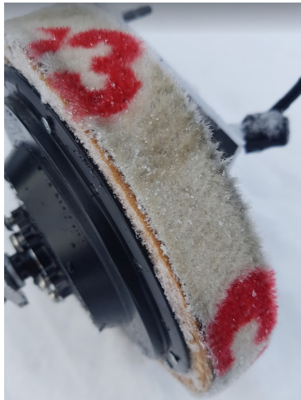
Figure 5.11: Skins attached on a drive wheel, after experiencing wheelspin.
