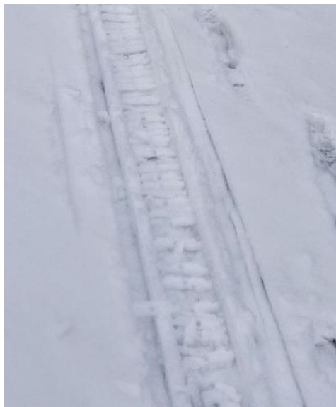
Figure 10: The track left in the snow by the prototype without the weight of the user.
