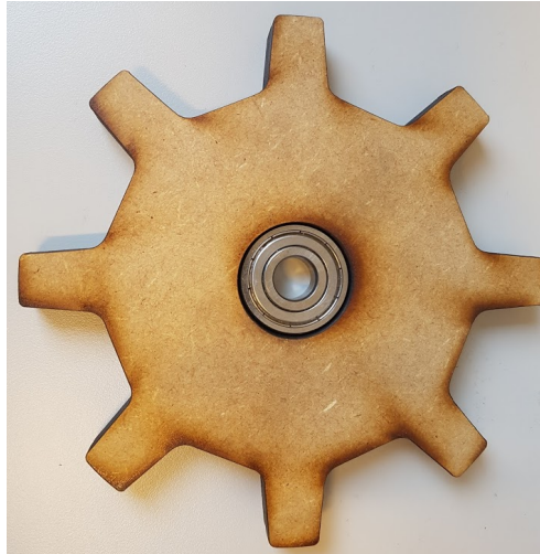
Figure 5.7: To rapidly make a sprocket wheel in exact dimensions, MDF-plates were laser cut and assembled on two parallel bearings.
