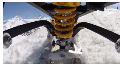
Figure 4.5: Tempo Dualski by Tessier with closer look at the tilt enabling mechanism [53].
