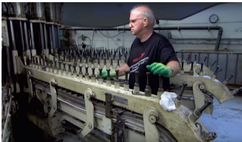
Figure 4.7: Madshus' adjustable ski mold [56].
