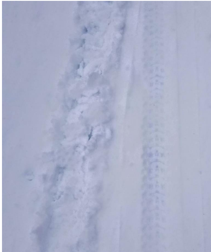
Figure 13: The tire tracks left on the ski trail from two different drive wheels on the same conditions; test 1 and 2.
