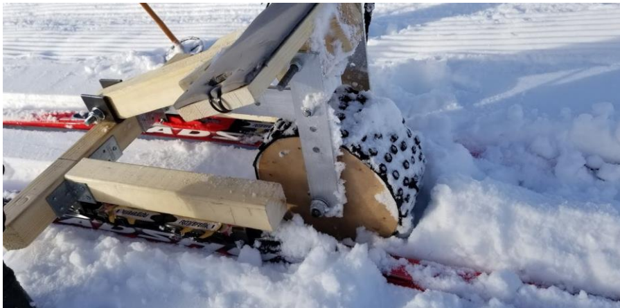
Figure 9: The small wheel prototype and effect of wheelspin on the new snow.
