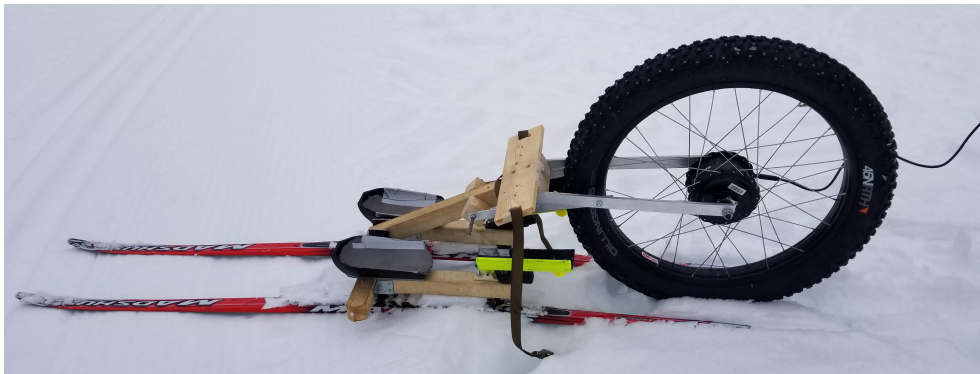
Figure 6.5: The chassis prototype with a different drive system, big wheel with fatbike tire.
