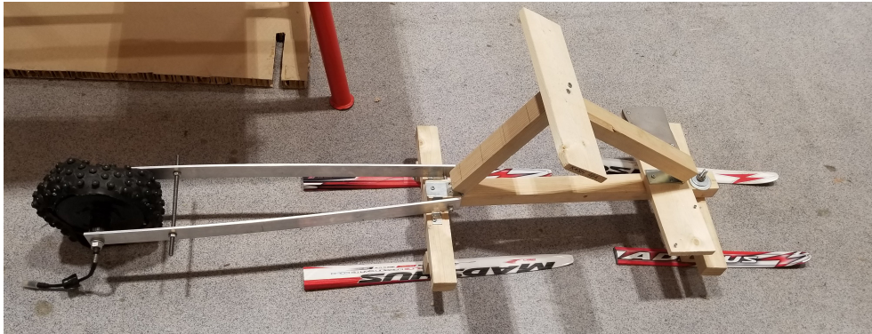
Figure 6.3: Chassis made to investigate magnitude of force required on the drive.
