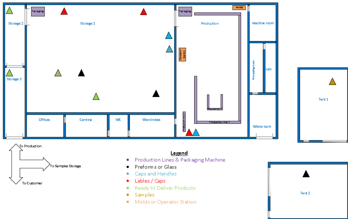
Figure 35: Current Facility Layout
