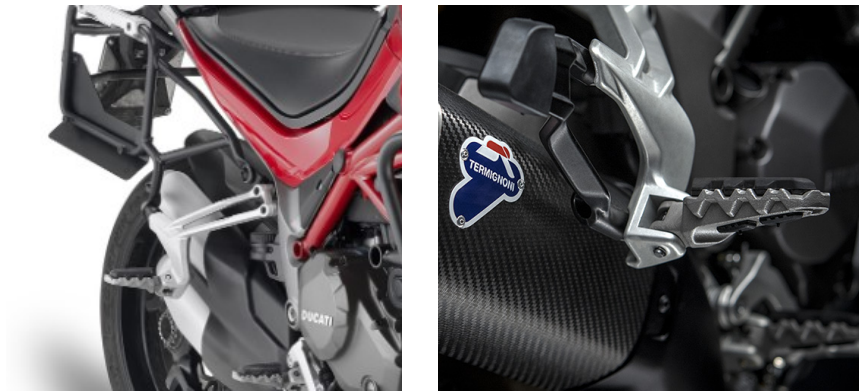
(a) Luggage rack mounted on the footpeg bracket [Carpimoto (2019)]. (b) Luggage support mounted on the footpeg bracket [Ducati (2019a)].
