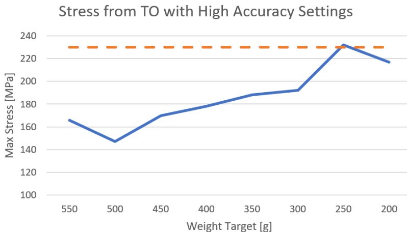
Figure 4.4: Max stress from different weight targets with high accuracy settings and orange yield limit.
