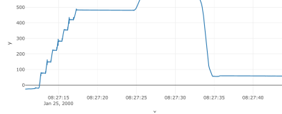
(b) Curve plot of the load applied to the torsion bar suspension rig for a given time series
