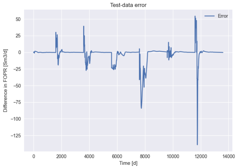
FIGURE 4.3: Error from the real test data from ECLIPSE minus the evaluation from the proxy model
