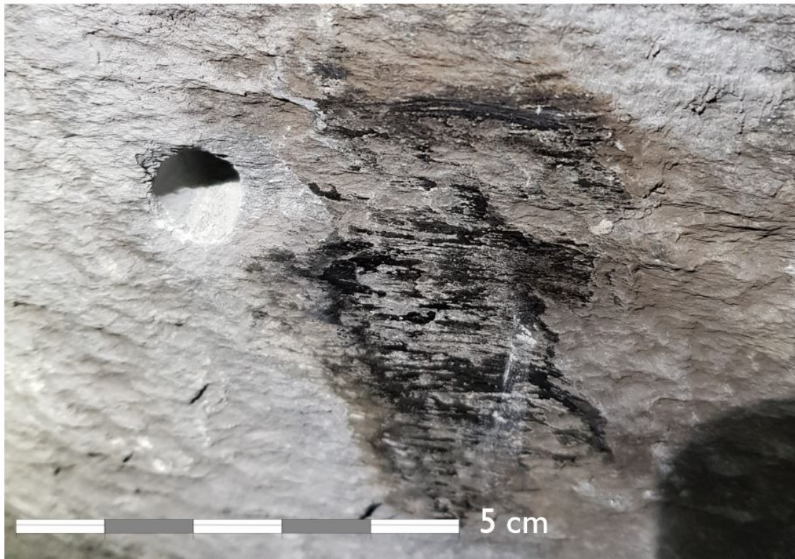
Figure 30: Flattened and smoothed area (black) after chiseling and angle grinding, this was done to ensure optimal coupling between the rock surface and AE sensors. (private photo).
