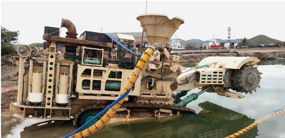
Figure 6 The Bulk Cutter during onshore function test [59].
