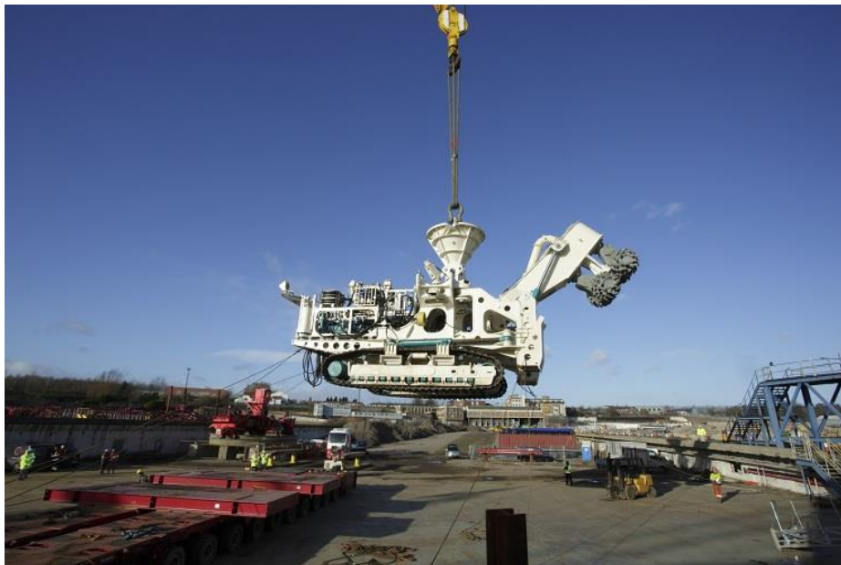
Figure 5 Auxiliary cutter. The primary "benching" cutter for leveling chimneys and flattening the production area [65]
