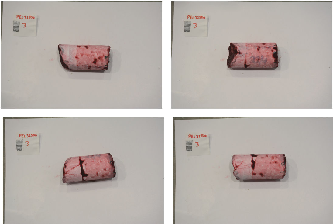
Figure 70: Dye penetrant test on sprayed concrete core 3 from profile number 32500.
