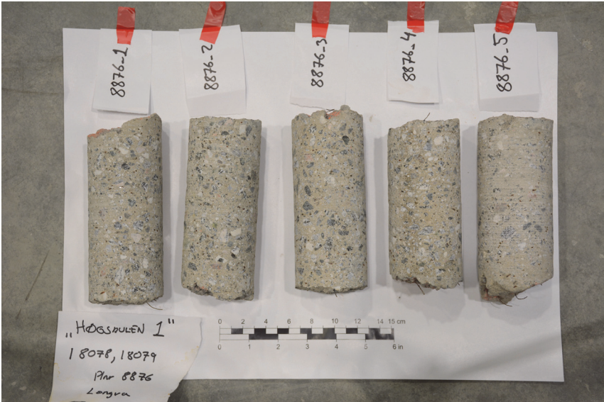
Figure 96: All the sprayed concrete cores from profile number 23903 in Longva before the testing.
