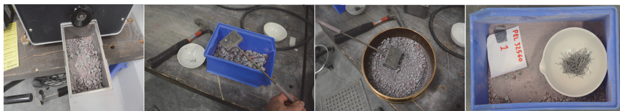
Figure 24: Method for crushing and separating the fibres from the cores.
