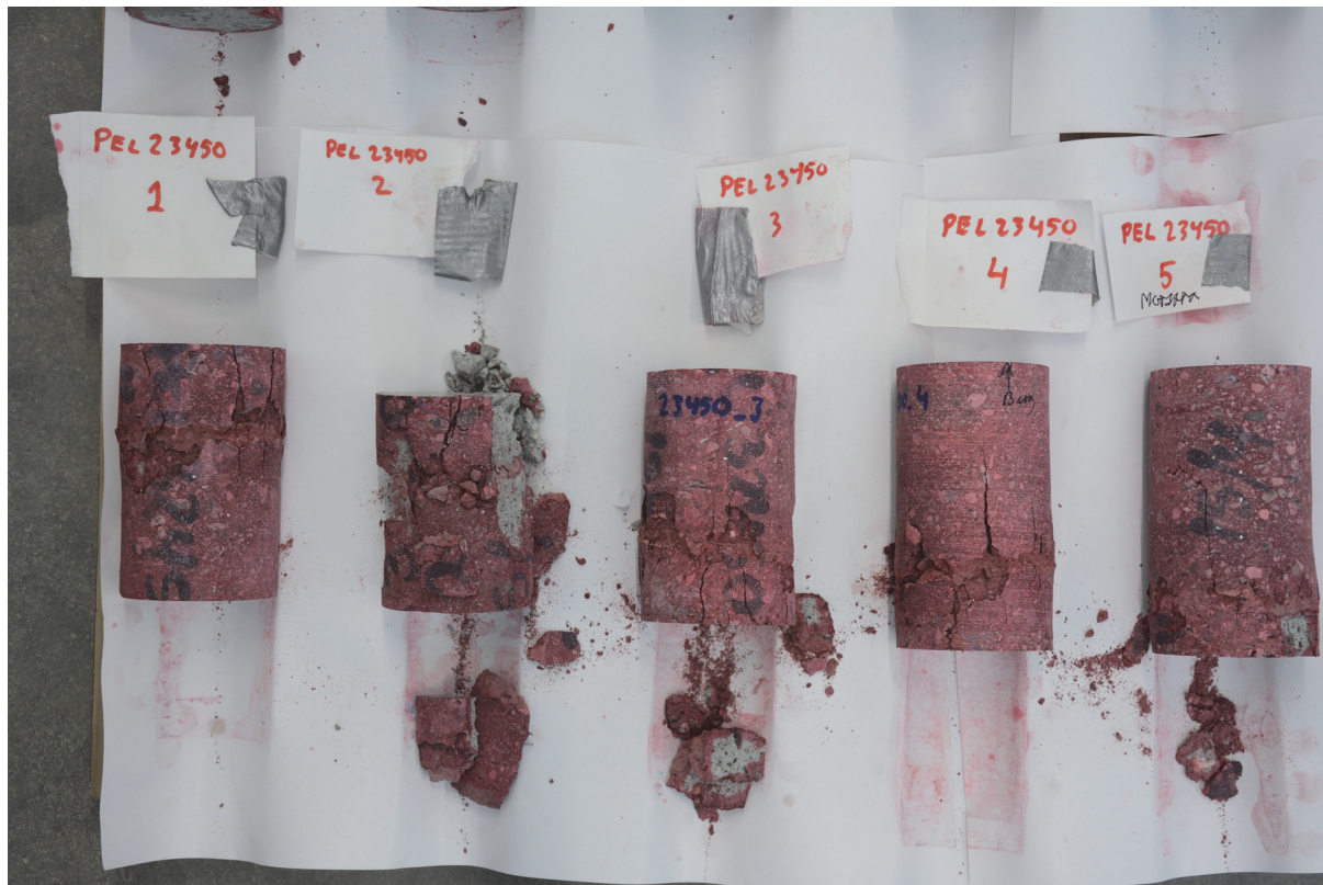
Figure 34: All cores from profile 32450 after compressive strength testing, with failure pattern along the boundary between two sprayed concrete layers.
