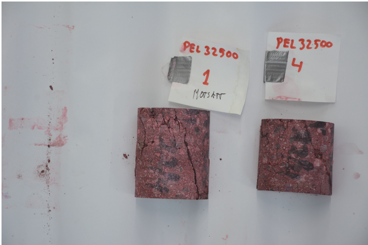
Figure 35: Two cores from profile 32500 after compressive strength testing, with failure patterns.
