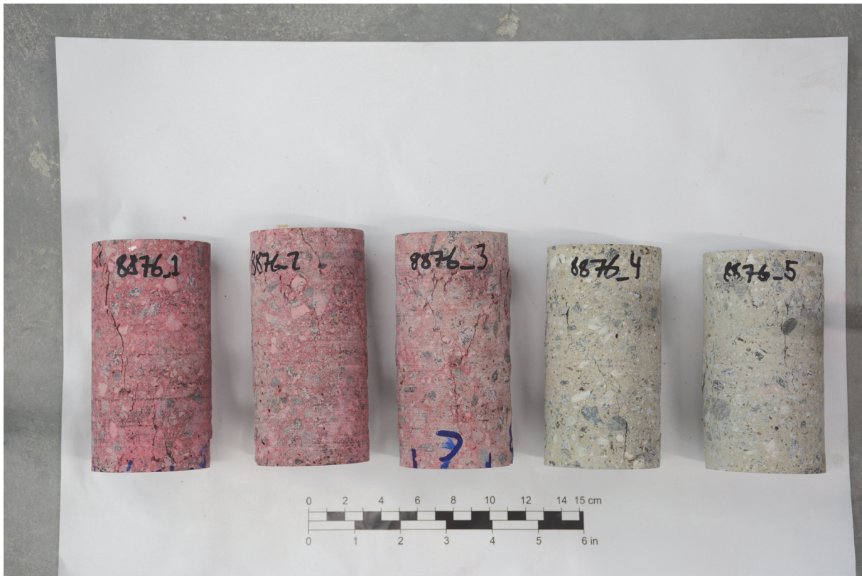
Figure 31: All cores from profile 23903 after compressive strength testing, with failure patterns.
