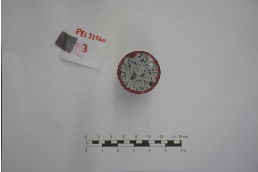
Figure 84: Penetration depth of dye on sprayed concrete core 3 from profile 32560.
