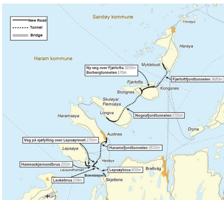
Figure 15: The planned route for Fv. 659 Nordøyvegen with tunnels and bridges. Taken from NPRA (2020a).
