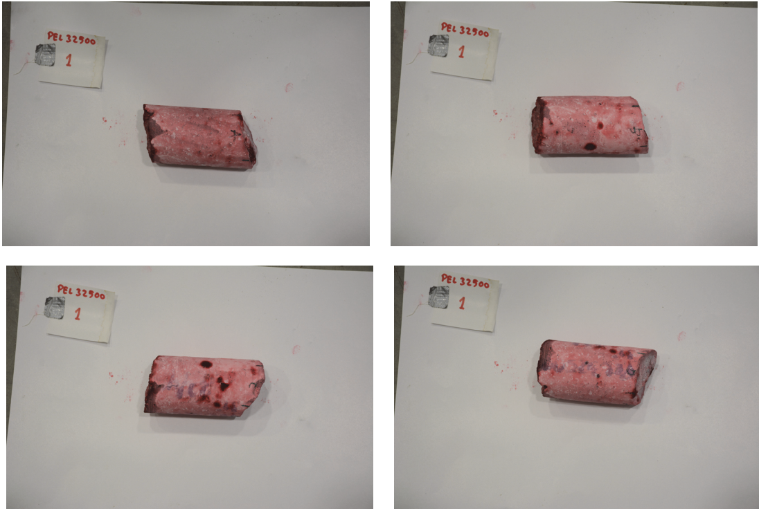
Figure 68: Dye penetrant test on sprayed concrete core 1 from profile number 32500.
