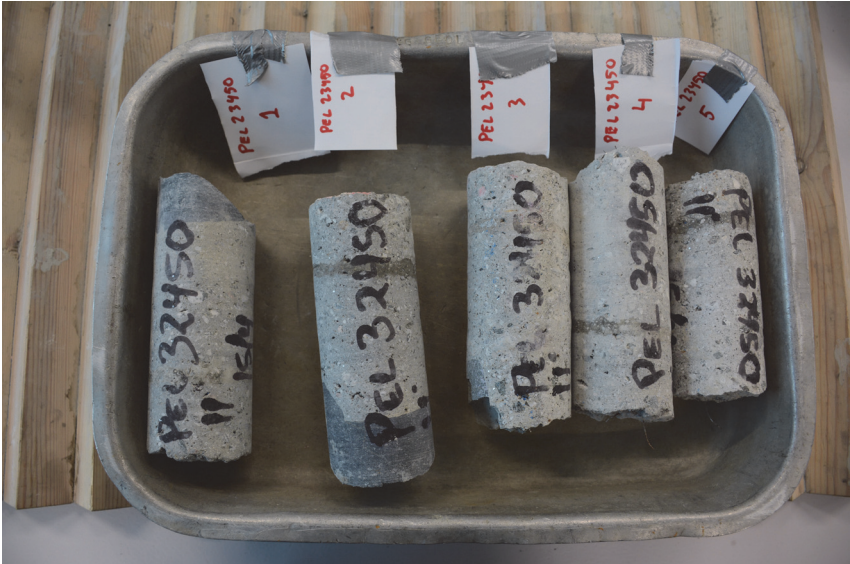
Figure 99: All the sprayed concrete cores from profile number 32450 in Fjørtofta before the testing.
