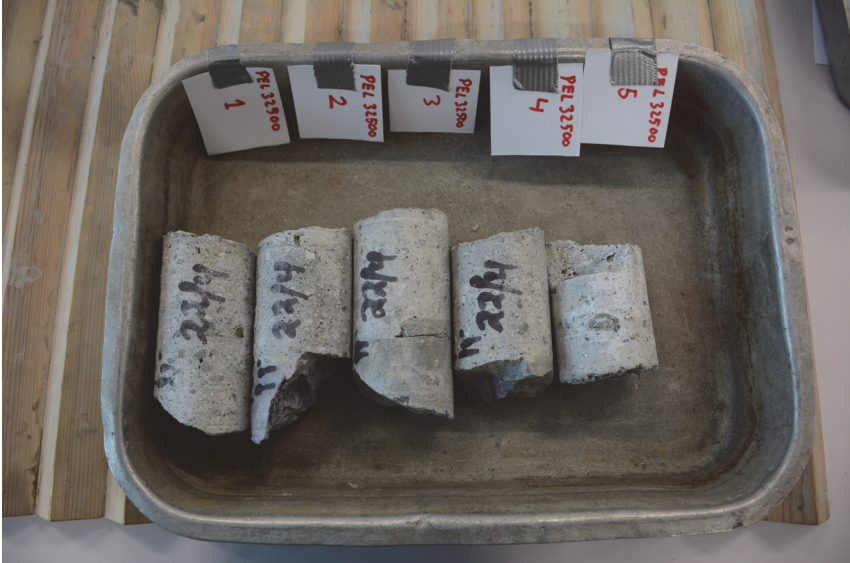
Figure 100: All the sprayed concrete cores from profile number 32500 in Fjørtofta before the testing.
