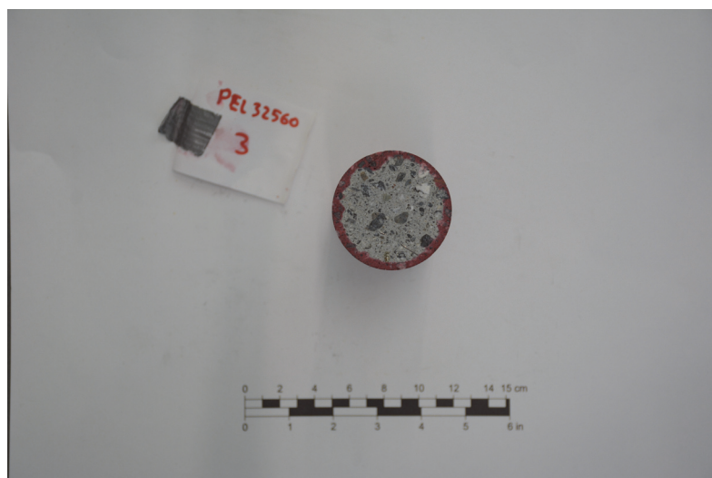
Figure 28: Penetration depth of dye on sprayed concrete core 3 from profile 32560.
