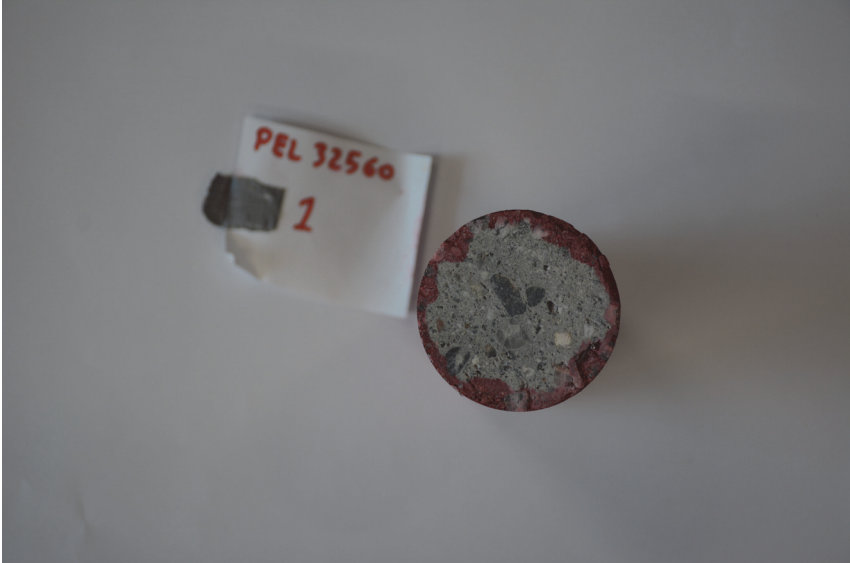
Figure 82: Penetration depth of dye on sprayed concrete core 1 from profile 32560.
