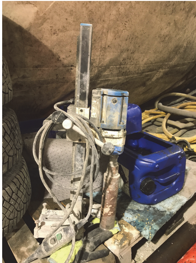
Figure 19: Boring machine, Shibuya TS-92, used to get the sprayed concrete samples.
