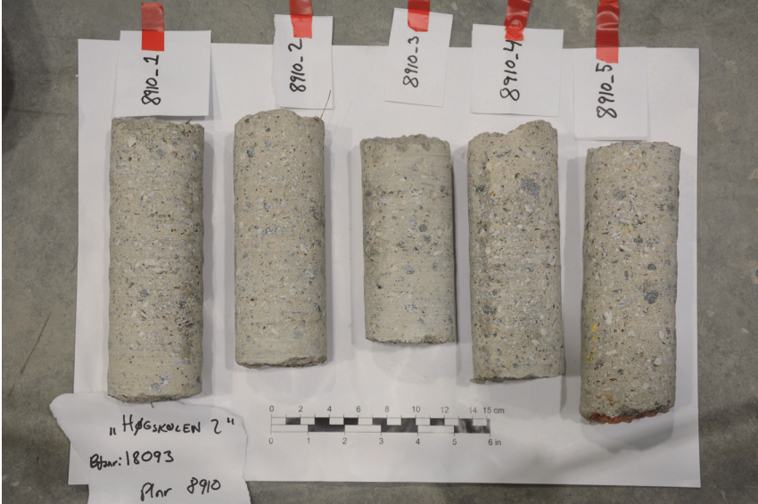
Figure 98: All the sprayed concrete cores from profile number 23917 in Longva before the testing.
