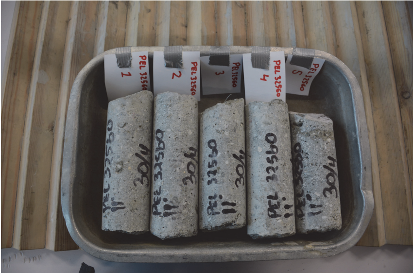
Figure 101: All the sprayed concrete cores from profile number 32560 in Fjørtofta before the testing.
