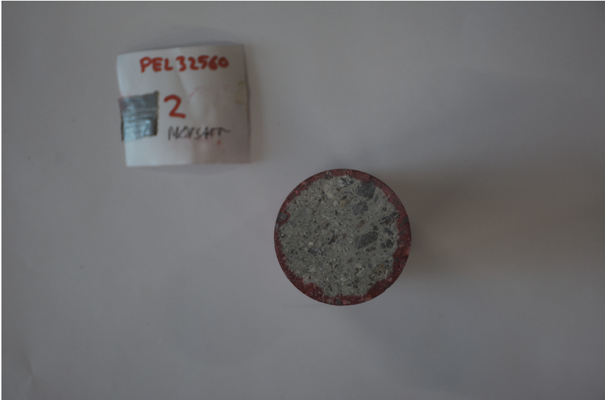
Figure 83: Penetration depth of dye on sprayed concrete core 2 from profile 32560.
