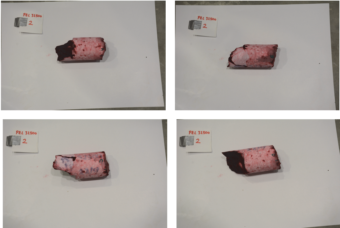
Figure 69: Dye penetrant test on sprayed concrete core 2 from profile number 32500.
