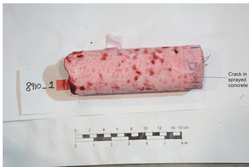
Figure 26: Dye penetrant crack mapping on sprayed concrete core nr. 1 from profile number 23917 with an arrow showing the crack on the core.
