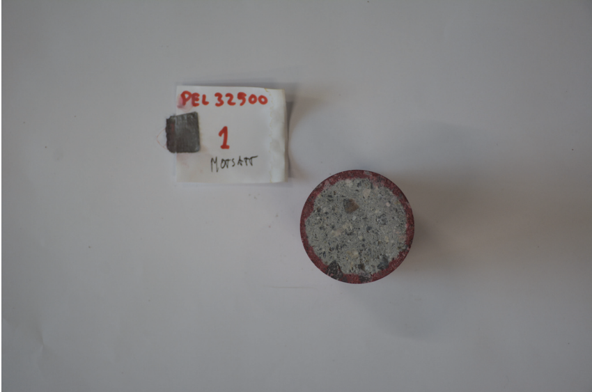
Figure 80: Penetration depth of dye on sprayed concrete core 1 from profile 32500.
