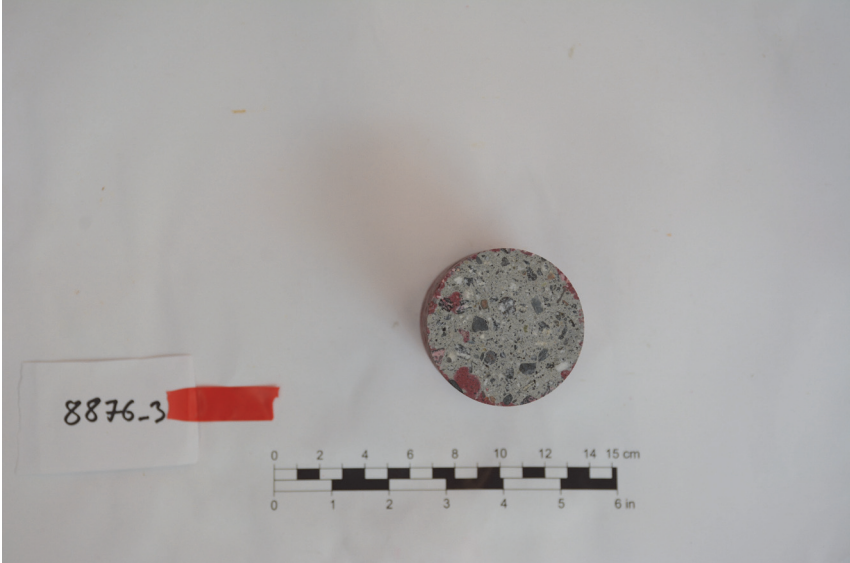
Figure 78: Penetration depth of dye on sprayed concrete core 3 from profile 23903.
