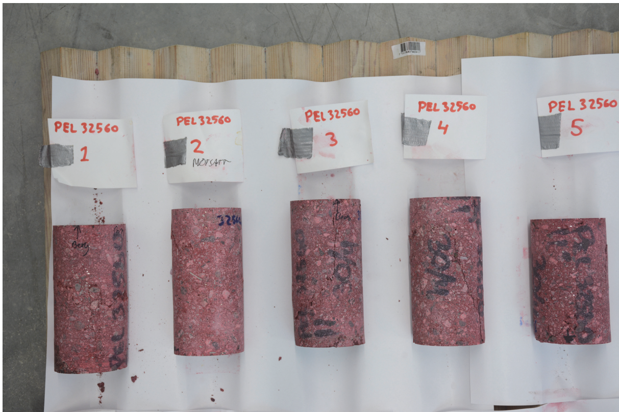
Figure 36: All cores from profile 32560 after compressive strength testing, with failure patterns.
