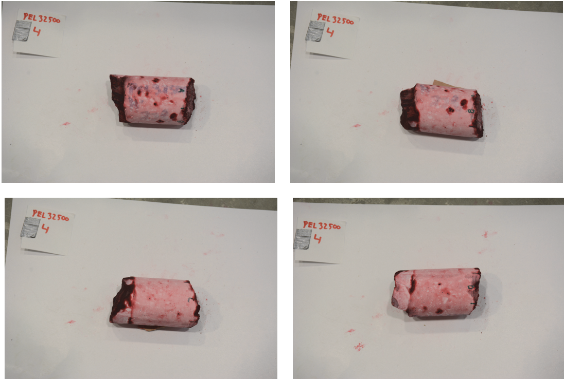
Figure 71: Dye penetrant test on sprayed concrete core 4 from profile number 32500.
