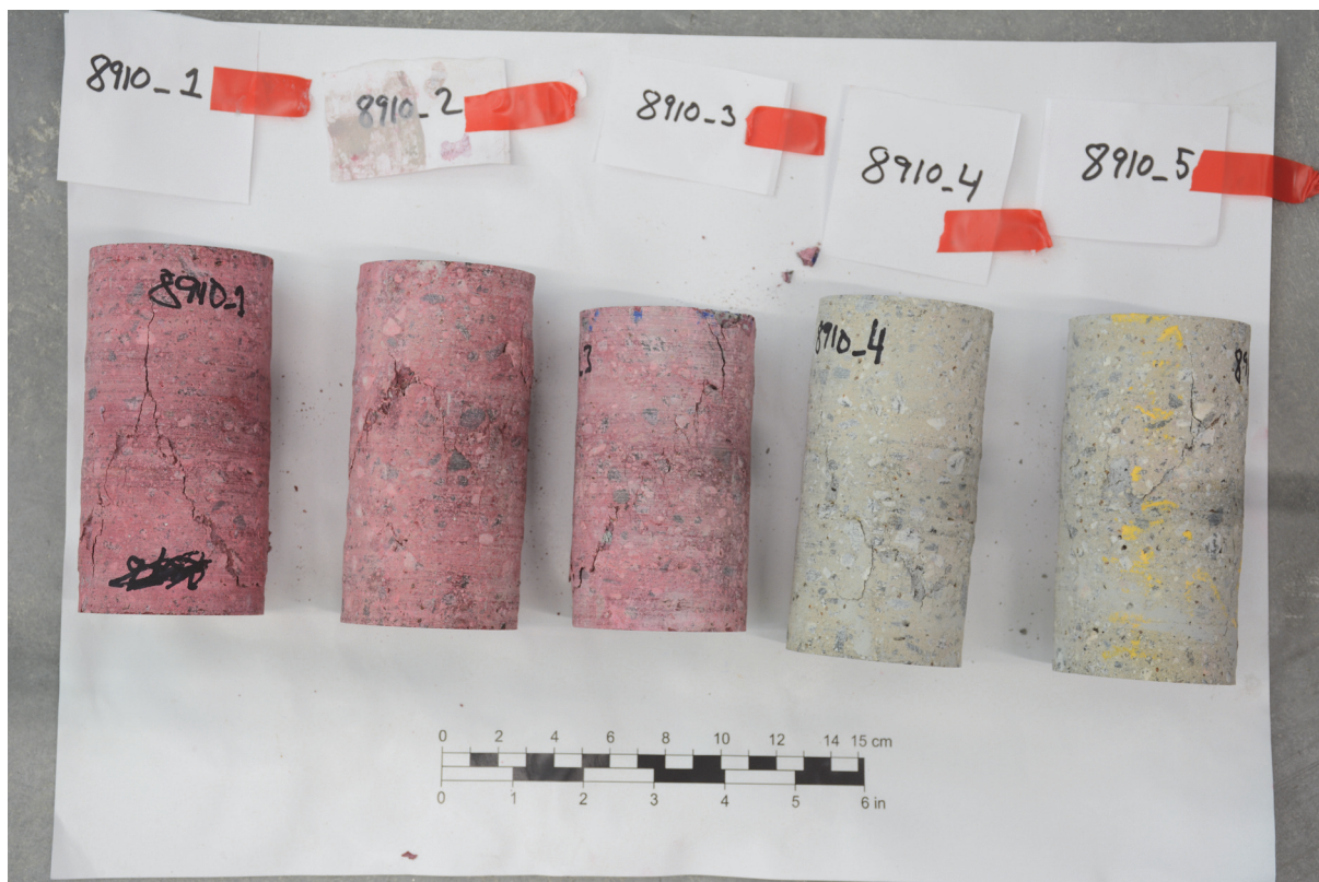
Figure 33: All cores from profile 23917 after compressive strength testing, with failure patterns.
