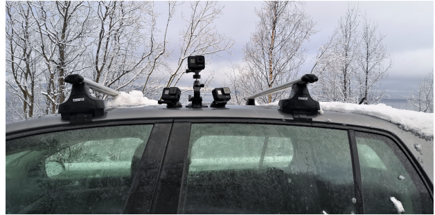
Figure 3.4: The three Gopro cameras were mounted on a car, collecting photos every 0.5 seconds while driving at a speed of 15-20 km/h along the rock cut.
