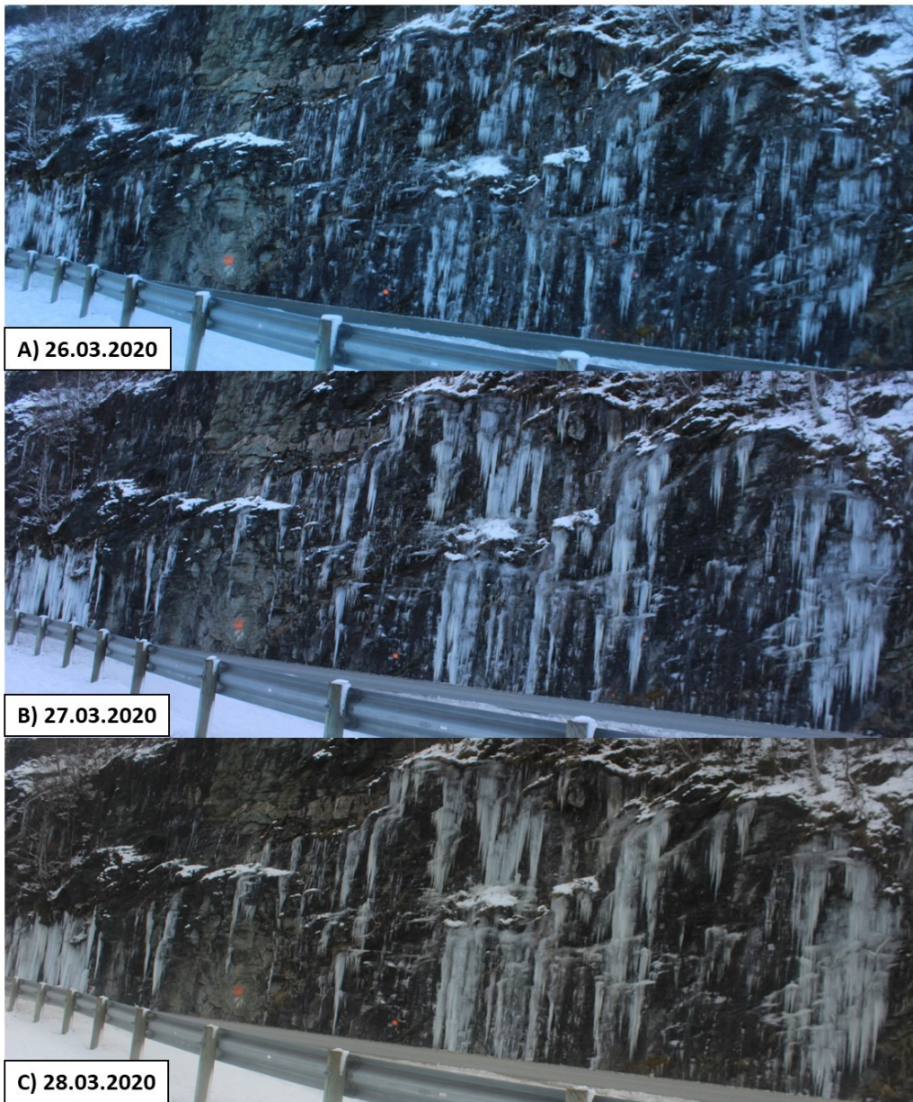
Figure 4.8: Temperatures dropped below 0^{\circ}\text{C} on February 25th, with ice starting to form rapidly after. Figure A, B and C show the progress during the 26th, 27th and 28th. The initial growth consists of the formation of a thin ice crust on the rock, and icicles extending continuously. On the 28th some icicles have reached the ground and have started forming ice columns. The boundaries of the ice was mapped by color recognition on the 28th. The previous days the color contrast of the ice and the rock was not suitable for mapping.
