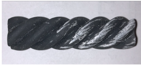
Figure C.3: First prototype of 3D-printed PDM rotor.
