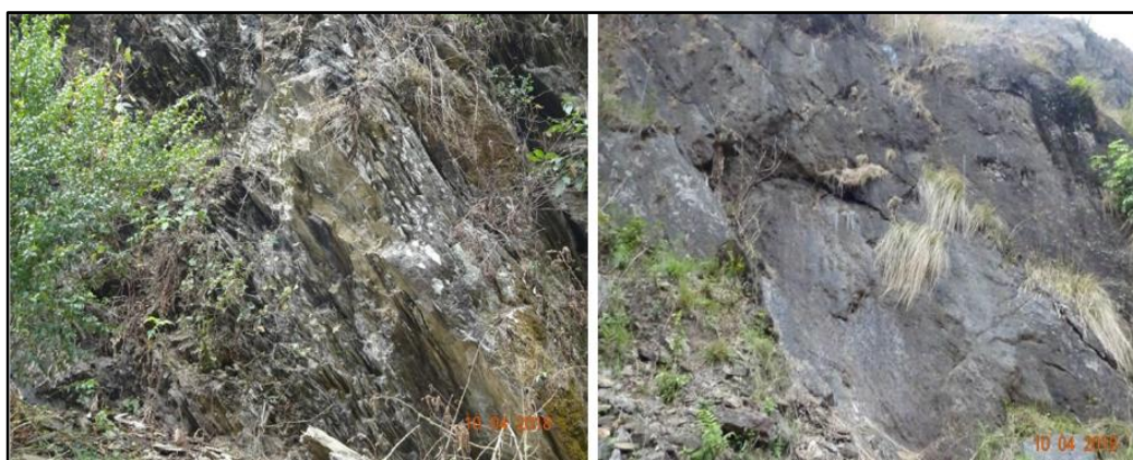
Figure 4-6 Rock mass quality in the project area: weak rock mass (left) and very strong rock mass (right) (NEA 2019)
