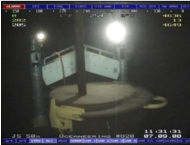
Figure 10: SMO mud level monitored by cameras and lights (Smith et al. 2010)
